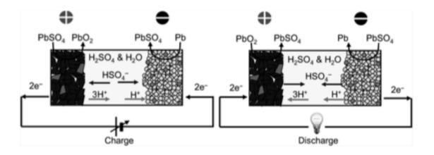
Figure 10. Principles of operation of a lead-acid battery Retrieved from (Glaize & Genies, 2012)
