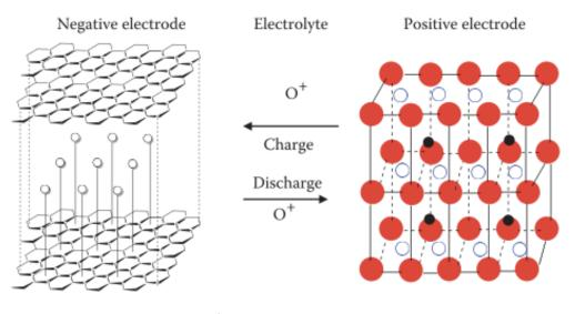
○: Atomic-state lithium O<sup>+</sup>: Solvated lithium ions •: Ionic-state lithium
