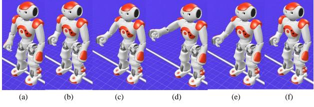
Figure 4.16 Forward reaching movements performed/demonstrated by NAO
