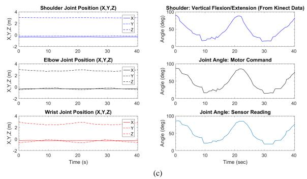
Figure 5.4 Shoulder joint flexion/extension teleoperation. (b) comparison between joint angles from Kinect and NAO robot.(c) coordinate data and joint angles from Kinect and NAO robot.
