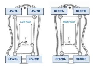
Figure 2.8 Force sensitive resistors(FSR) location on the feet of NAO (SoftbankRonotics,2013)
