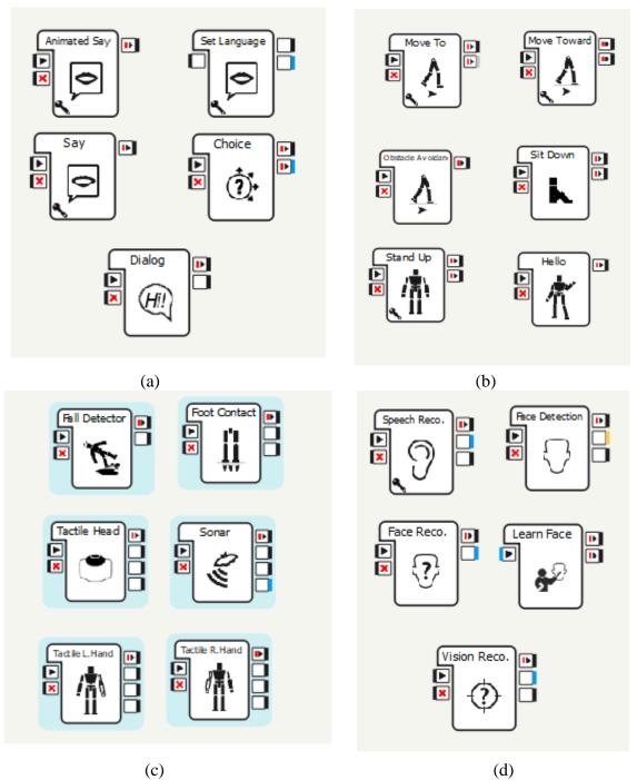
Figure 4.3 Functions blocks in Choregraphe. (a) Audio blocks, (b) Motion blocks, (c) Sensing blocks, (d) Intelligent blocks
