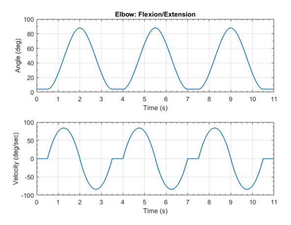
Figure .4.14 Elbow joint flexion/extension (joint trajectory and velocity)
