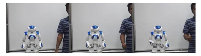
Figure 5.7 Arm position of human operator and NAO robot during elbow joint flexion/extension motion during teleoperation
