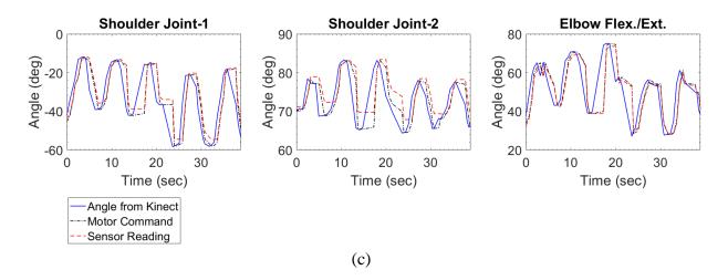
Figure 5.12 Diagonal reaching teleoperation. (a) Joint coordinate from Kinect (b) skeleton with joint coordinate from Kinect (c) comparison between joint angles from Kinect and NAO robot
