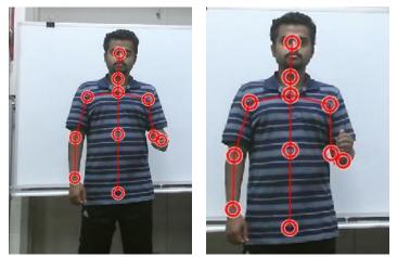
Figure 6.5 wrist and elbow joint tracked by Kinect sensor for same position.
