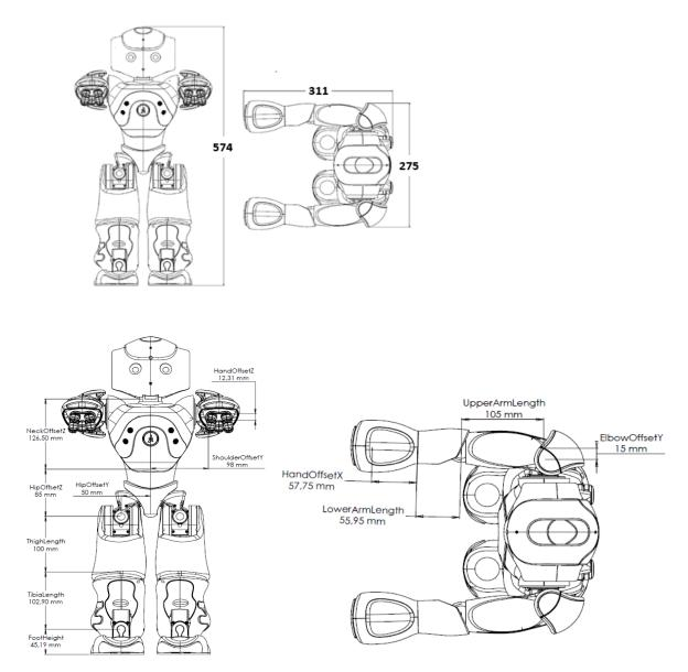
Figure 2.1 Dimensions of NAO robot
