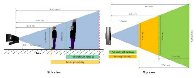
Figure 3.3 Field of view of Kinect sensor(Wiki)
