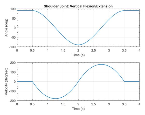
Figure 4.10 Shoulder joint vertical flexion/extension motion (fast movement)
