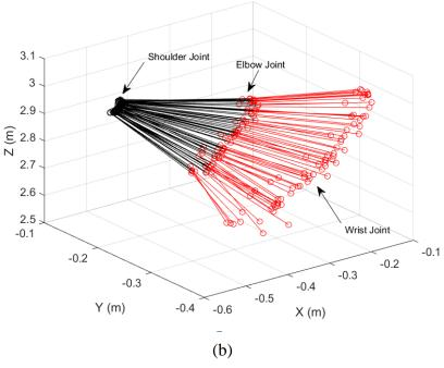
Shoulder Joint: Horizontal Flexion/Extension Motion (Kinect Data)
