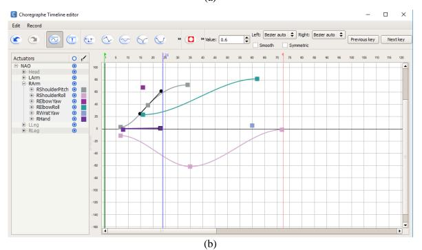
Figure 4.5 (a) Timeline block, (b) Motor trajectory control inside the timeline block
