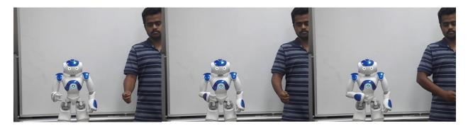
Figure 5.5 Arm position of human operator and NAO robot during shoulder joint Internal/external rotation during teleoperation
