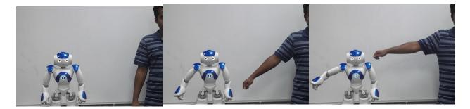
Figure 5.1 Arm position of the human operator and NAO robot during shoulder joint abduction/adduction teleoperation.
