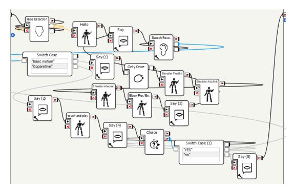
Figure 4.21 NAO's behavior programming for single and multi-joints movements and cooperative tasks
