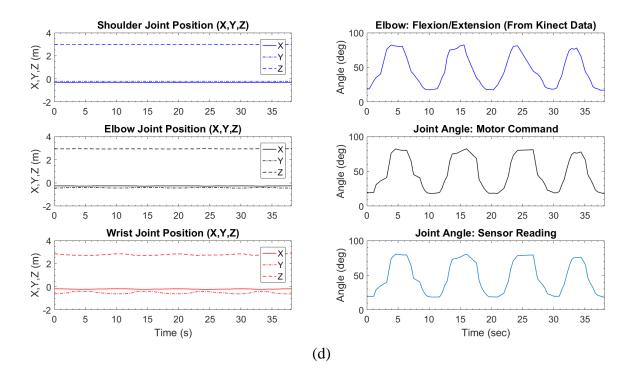
Figure 5.8 Elbow flexion/extension teleoperation. (a) Skeleton with joint coordinate from kinect(b) Joint coordinate from Kinect (c) comparison between joint angles from Kinect and NAO robot.(d) coordinate data and joint angles from Kinect and NAO robot.
