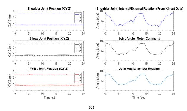
Figure 5.6 Shoulder joint internal/external rotation teleoperation. (a) Joint coordinate from Kinect (b) comparison between joint angles from Kinect and NAO robot.(c) coordinate data and joint angles from Kinect and NAO robot.
