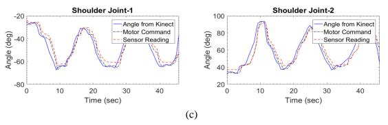
Figure 5.10 Shoulder joint horizontal flexion/extension teleoperation. (a) Joint coordinate from Kinect (b) skeleton with joint coordinate from Kinect (c) comparison between joint angles from Kinect and NAO robot.
