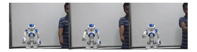
Figure 5.3 Arm position of human operator and NAO robot during shoulder joint vertical flexion/extension teleoperation
