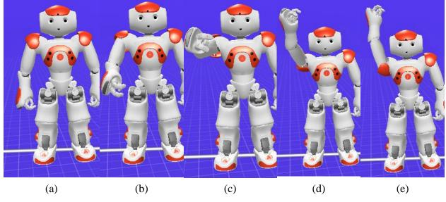
Figure 4.9 Shoulder flexion/extension motion of NAO.
