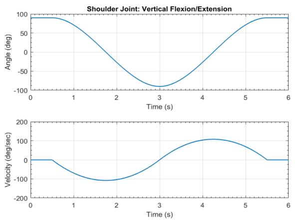
Figure 4.8 Shoulder joint vertical flexion/extension motion (joint trajectory and velocity)
