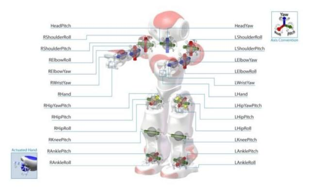
Figure 2.2 All joints in NAO robot (SoftbankRonotics,2013)
