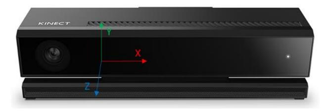
Figure 3.1 Kinect sensor(Microsoft 2017)
