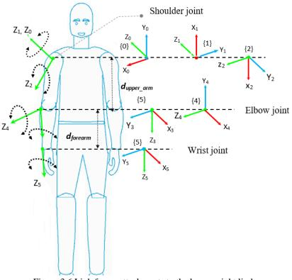
Figure 3.6 Link frame attachments to the human right limb
