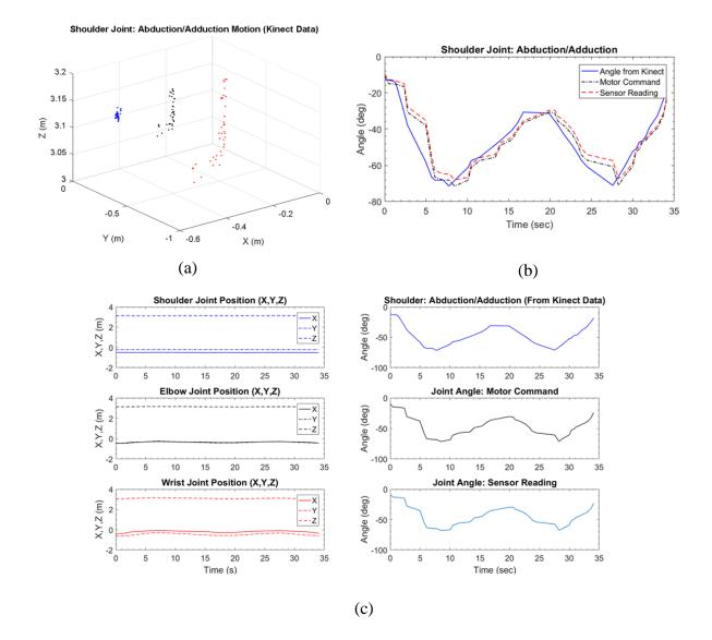
Figure 5.2 Shoulder joint abduction/adduction teleoperation. (a) Joint coordinate from Kinect (b) comparison between joint angles from Kinect and NAO robot.(c) coordinate data and joint angles from Kinect and NAO robot.
