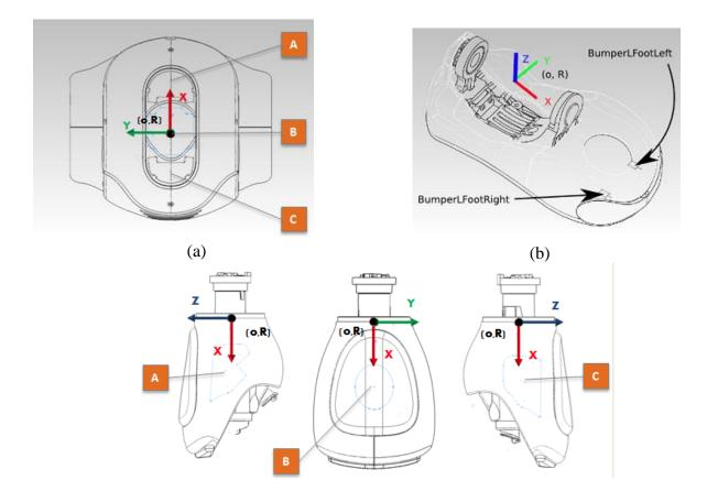
(a) tactile sensor position in head, (b) foot bumper position, (c) tactile sensor position in hand
