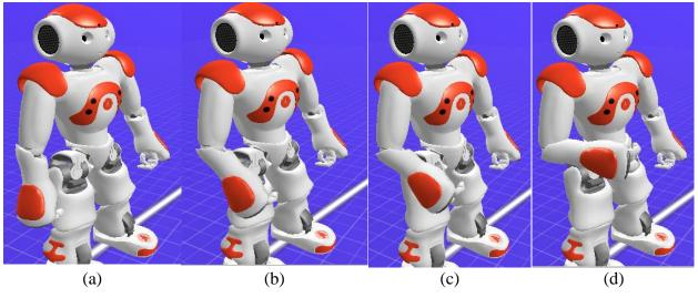
Figure 4.13 Elbow joint flexion/extension of NAO
