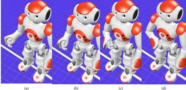
Figure 4.12 Shoulder joint internal/external rotation of NAO. (a) Elbow joint at ~90°, (b-d) internal/external rotation
