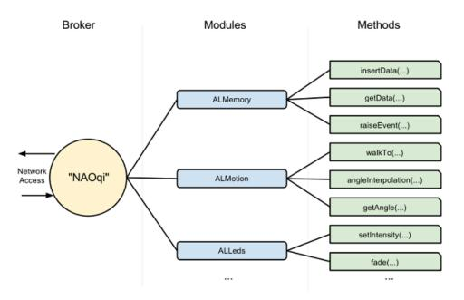
Figure 2.10 NAOqi work process
