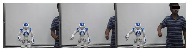
Figure 5.11 Arm position of human operator and NAO robot for Diagonal reaching motion during teleoperation Diagonal Reaching Movement (Kinect Data)
