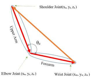
Figure 4.7 joint angle  $\theta_4$  calculation
