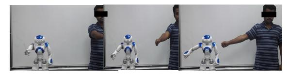
Figure 5.9 Arm position of human operator and NAO robot during Shoulder joint horizontal flexion/extension motion during teleoperation
