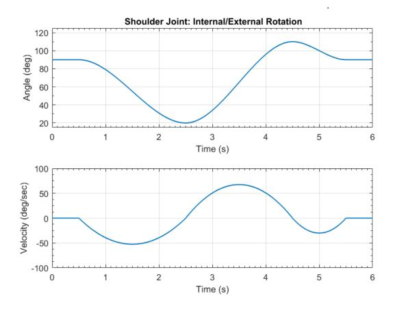
Figure 4.11 Shoulder joint internal/external rotation (joint trajectory and velocity)
