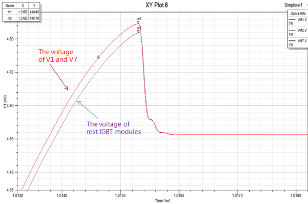
Figure 4-21 The resistance of V1 and V7 is 0.1mΩ greater than others-voltage comparison of module MOV mode
