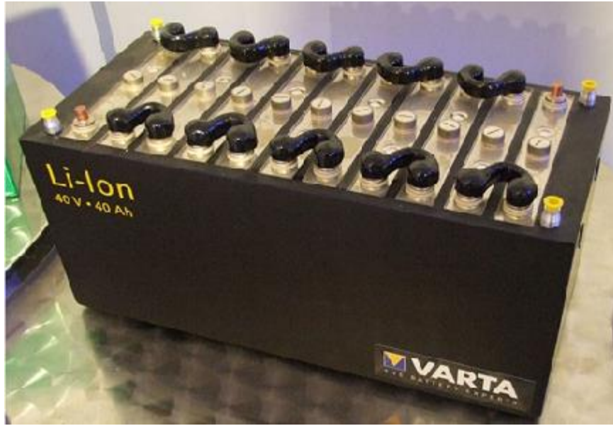
Figure 3.1. Typical initial Lithium ion battery pack
