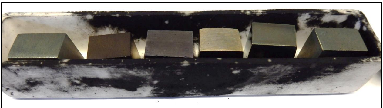
Figure 24. Photo of the crucible with samples after coking with CO CO-CO 2 -H 2 O at 600 °C for 169 h
