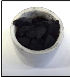
Figure 27. Carbon deposited during C_2H_6 atmosphere at 850 C for 100 hours
