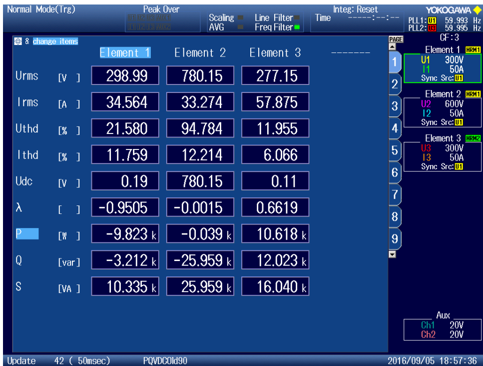
Figure 116 - Measurements of "PQ" Consuming 0.57 pu Active and 0.57 pu Reactive Power at 4500Hz
