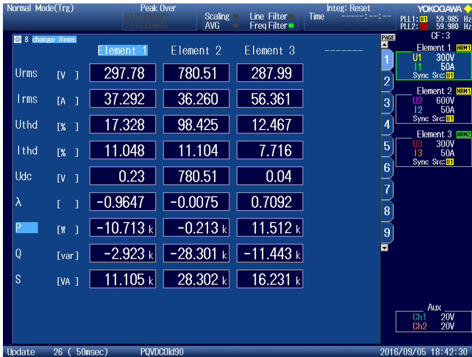
Figure 118 - Measurements of "PQ" Consuming 0.57 pu Active and Supplying -0.57 pu Reactive Power at 4500Hz
