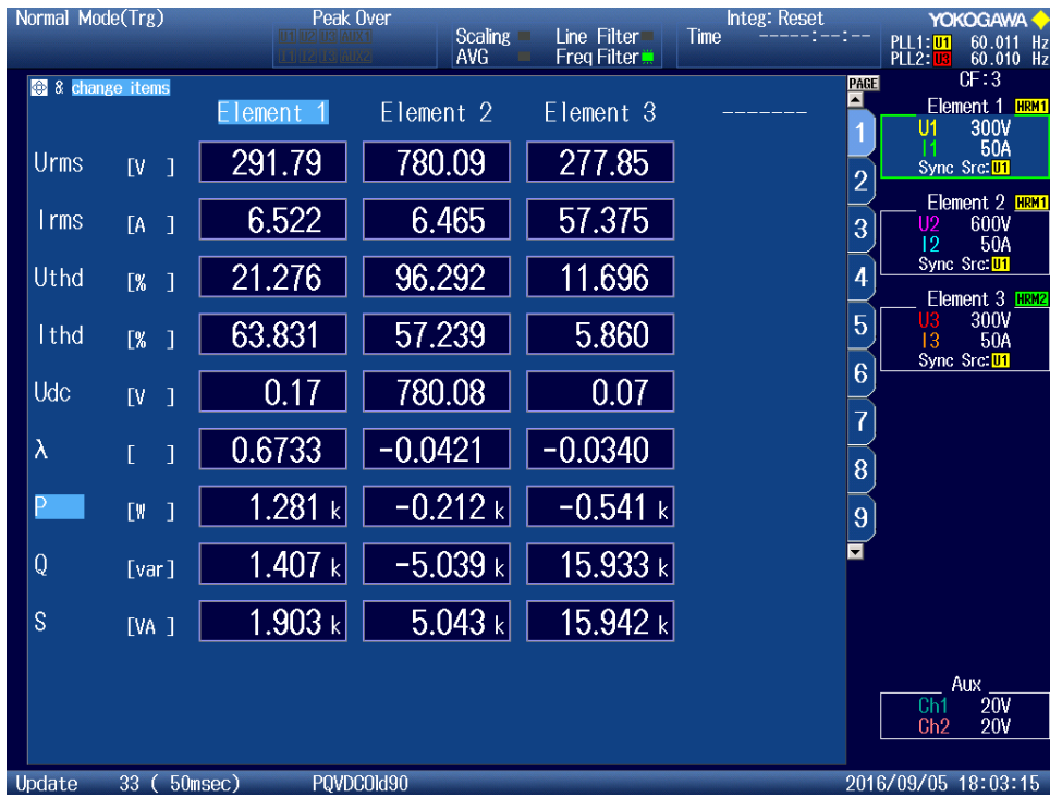
Figure 114 - Measurements of "PQ" Consuming 0.8 pu Reactive Power at Inductor Operation at 4500Hz
