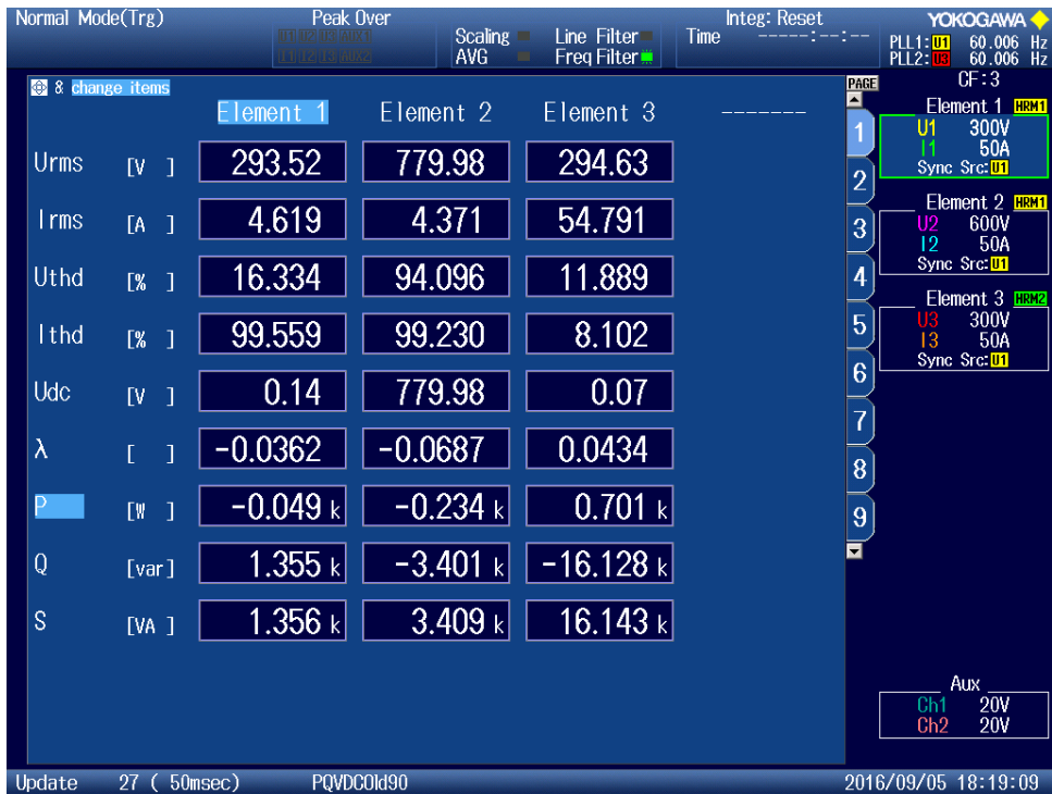
Figure 112 - Measurements of "PQ" Supplying -0.8 pu Reactive Power at Capacitor Operation at 4500Hz
