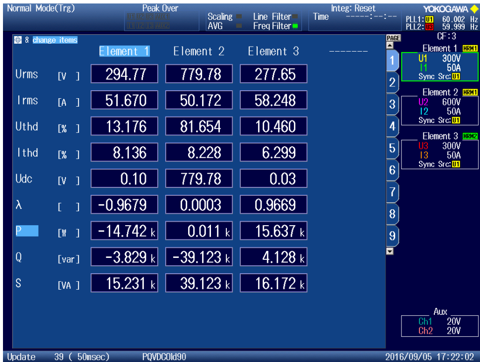
Figure 110 - Measurements of "PQ" Consuming 0.8 pu Active Power at Unity Power Factor at 4500Hz
