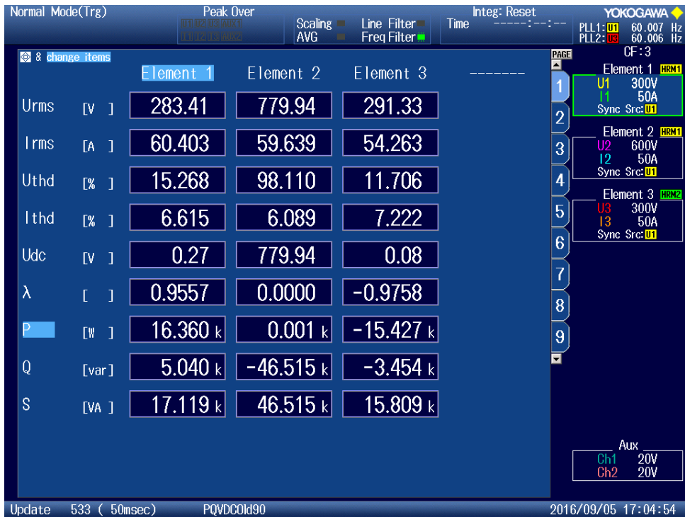
Figure 108 - Measurements of "PQ" Supplying -0.8 pu Active Power at Unity Power Factor at 4500Hz
