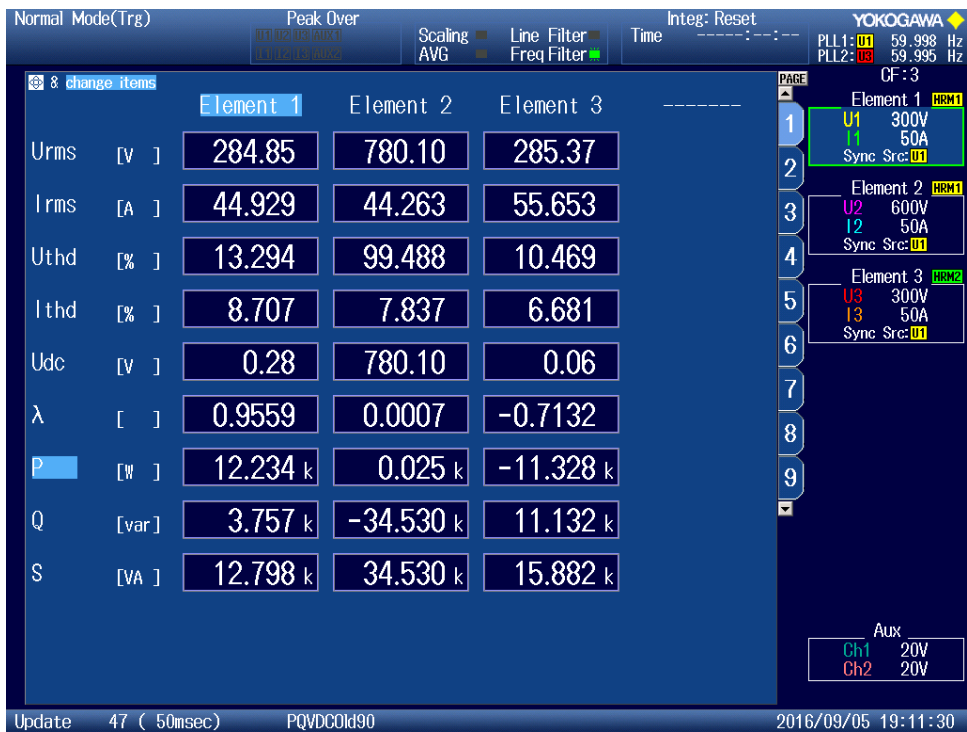
Figure 122 - Measurements of "PQ" Supplying -0.57 pu Active and Consuming 0.57 pu Reactive Power at 4500Hz
