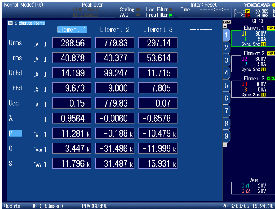
Figure 120 - Measurements of "PQ" Supplying -0.57 pu Active and -0.57 pu Reactive Power at 4500Hz
