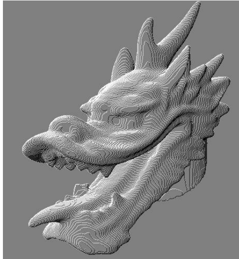
Figure 4.5: Visual representation of gradient directions of the scene input. To note are the contours formed by “layers” at the same directions.
