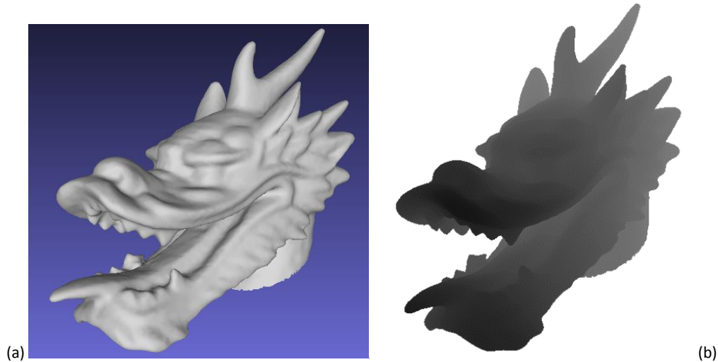
Figure 4.1: The dragon head is used as the sample input: (a) The original mesh (b) The generated depth map.
