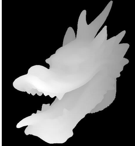
Figure 4.2: The depth map after non-linear compression. The background is still distant in this example. The depth measure is also inverted to fit with the convention of larger intensity representing larger heights.
