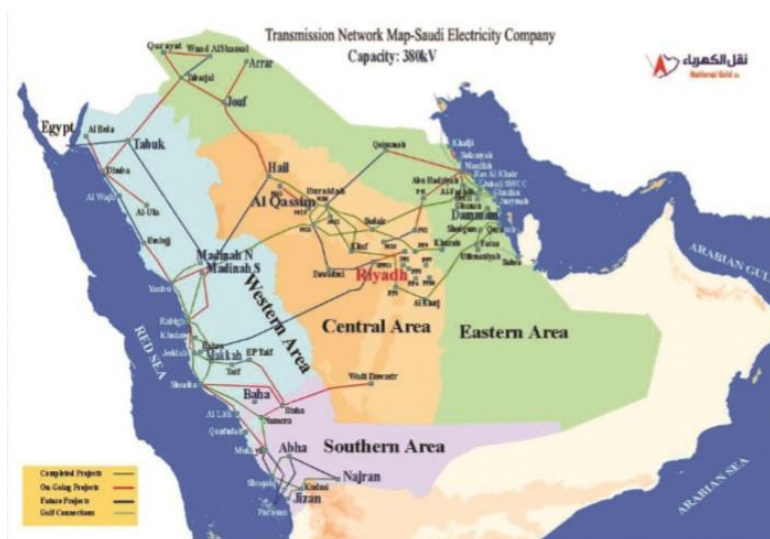
[Figure 4: Transmission Network Map, SEC Electrical Data 2000-2014]
