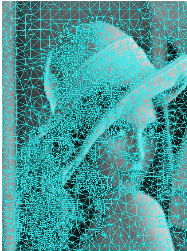
Fig 2.2: Initial triangle mesh generated by Delaunay triangulation.
