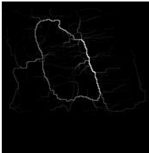
Figure 5.6: The edge confidence (EC) map formed by adding one to pixels where a shortest path goes through.
