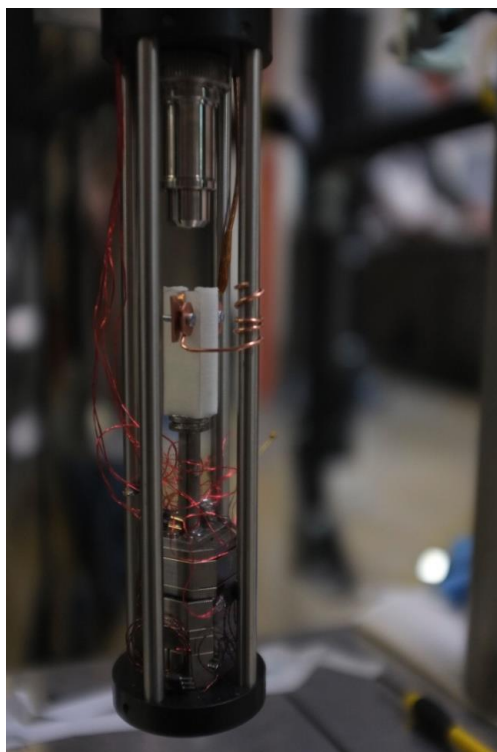
Figure 7.2: Left: Sample cell attached at the base of the optical insert of the CTCSM. The low dielectric properties of the DuraForm PA provide for insulation between the high voltage at the electrodes and the piezo positioners upon which the sample cell sits just below the CTCSM objective. The electrical connections consist of the Kapton insulated voltage carrying lead at the far electrode, and the semi-rigid grounding connection (thick copper wire) which provides for additional positional stability of the affixed sample cell at the front electrode. Right: Close-up of dual channel sample cell with 1 mm electrode spacing. Cover glass is placed atop sample and slides into sample cell. The edge of the cover glass can be seen on the left side of the image.
