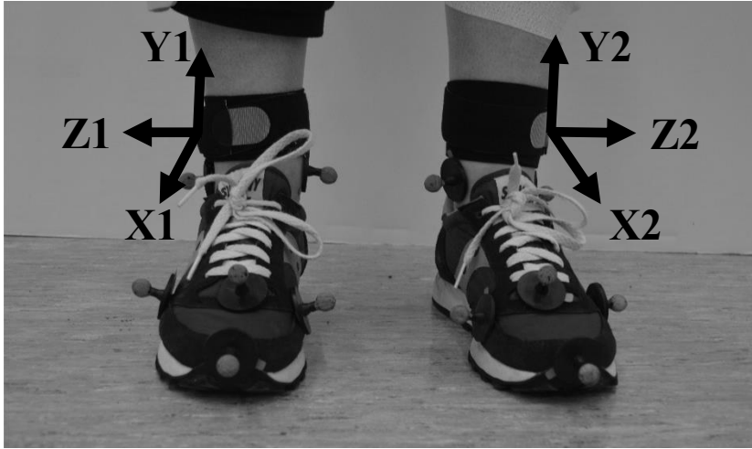
Figure 15. Orientation of the axes for each accelerometer.
