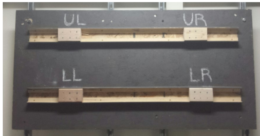
Figure 11: Hammering board setup with four reach positions
