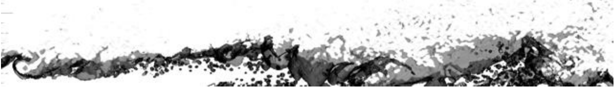
Figure 6-13 Normal water surface tension simulation (0.074N/m) with V_{air}=40m/s (Time interval = 10 msec)
