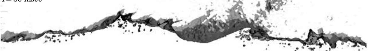
Figure 6-9 Normal water surface tension simulation (0.074N/m) with V_{air}=20m/s (Time interval = 10 msec)
