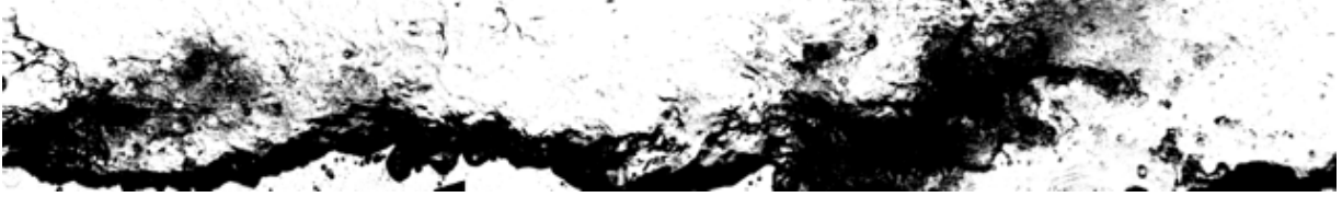
Figure 5-5 Normal water surface tension (0.074N/m) with V_{air}=40m/s (Time interval = 10 msec)
