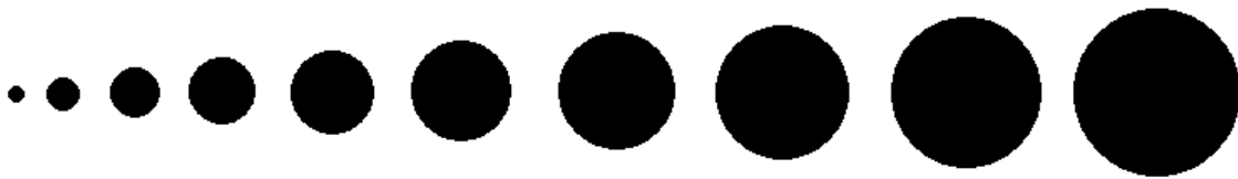
Figure 3-2 Test image with 10 different size from 10 to 100 pixels with increment of 10 pixel
