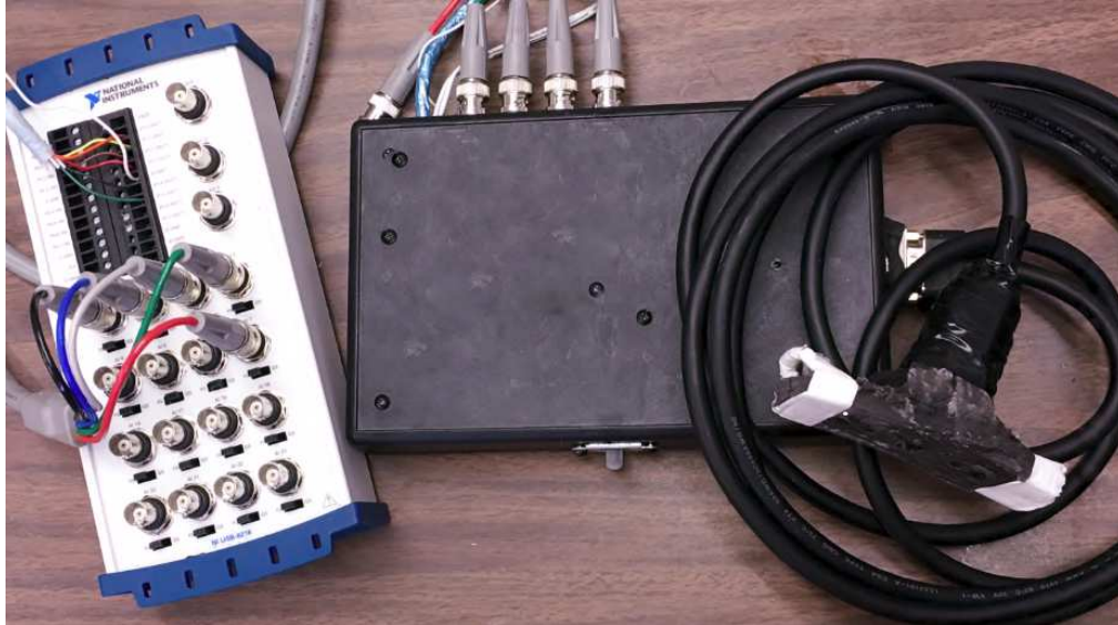
Figure 2.3 The DAQ board control box and probe of the oximetry hardware
