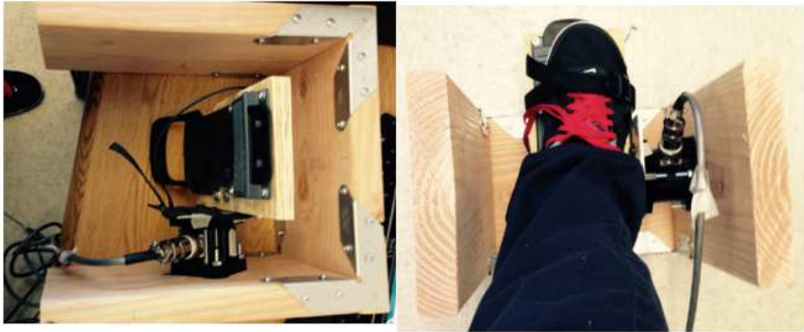
Figure 2.10 The Foot restraint apparatus. This apparatus is designed to hold the strain gauge upright and on any side while allowing the subjects foot to access to the strain gauge.
