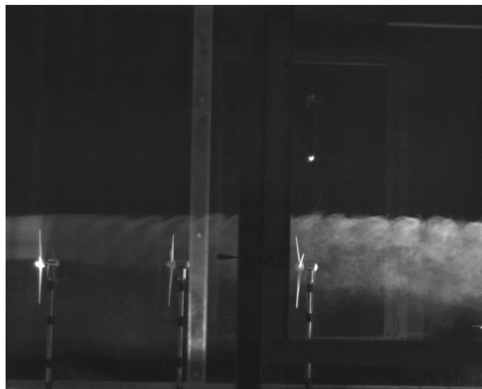
Figure 6-33. High speed image showing wake vortex and turbulence from three turbines spaced 2 rotor diameters apart
