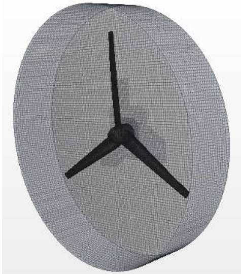
Figure 7-5. Rotating subdomain using trimmed mesh model with prism layer meshing at rotor surfaces
