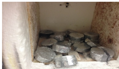
Figure 26 The mixed powders pressed into pellets using formed cylindrical pellets
