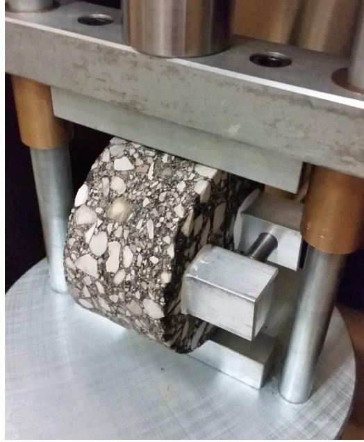
Figure 4.21 Complete Testing Setup for Fatigue
