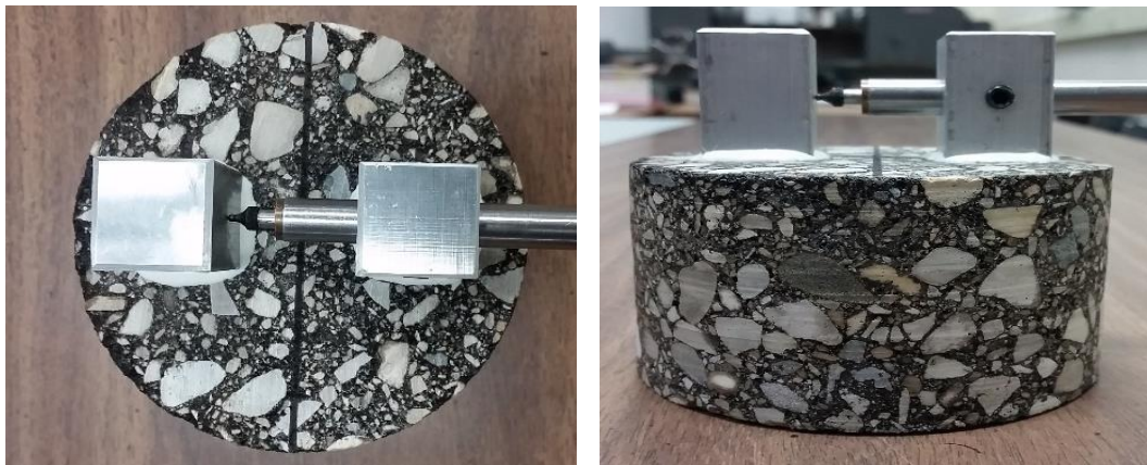
Figure 4.20 Asphalt Sample Assembly for Fatigue Testing
