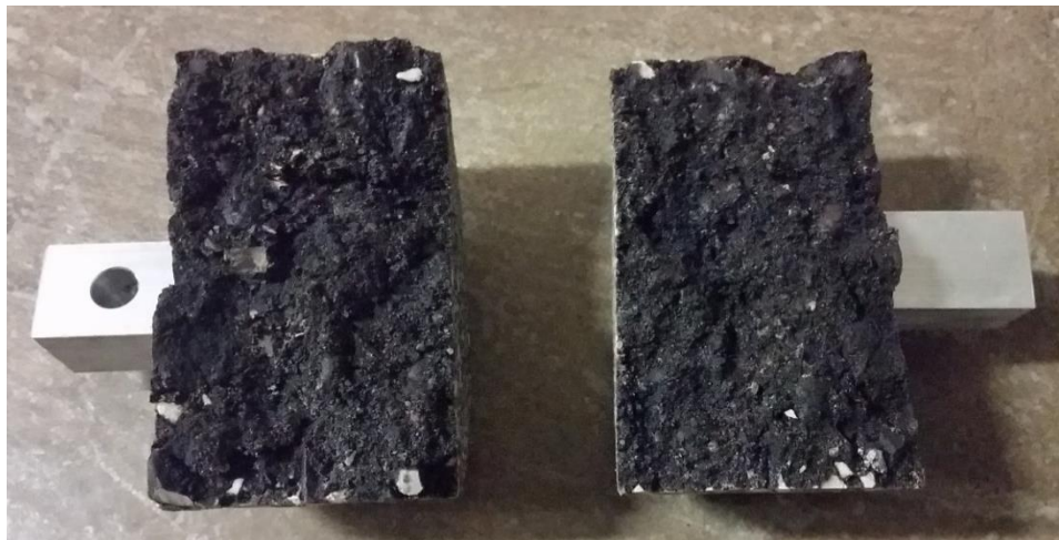
Figure 5.14 Representative Sample Failed in Fatigue
