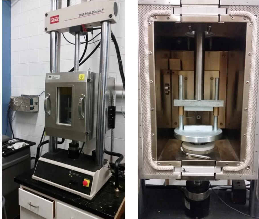
Figure 4.18 MTS Environmental Chamber with IDT Testing Frame
