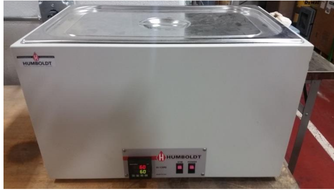
Figure 4.13 Humboldt Water Bath set at 60°C.
