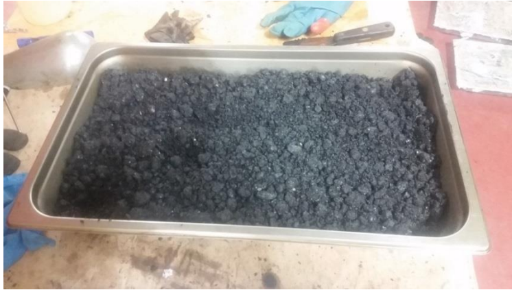
Figure 4.9 Compacted Asphalt Material after being Melted
