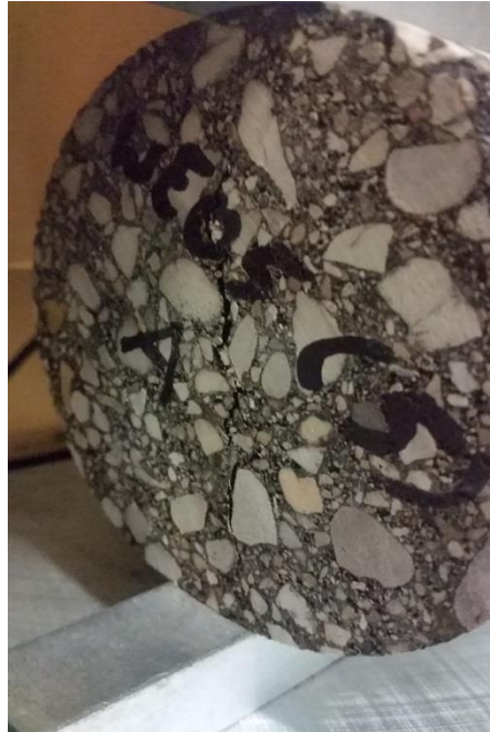
Figure 5.13 Fatigue Crack Propagating for a WE05 C 10% Sample
