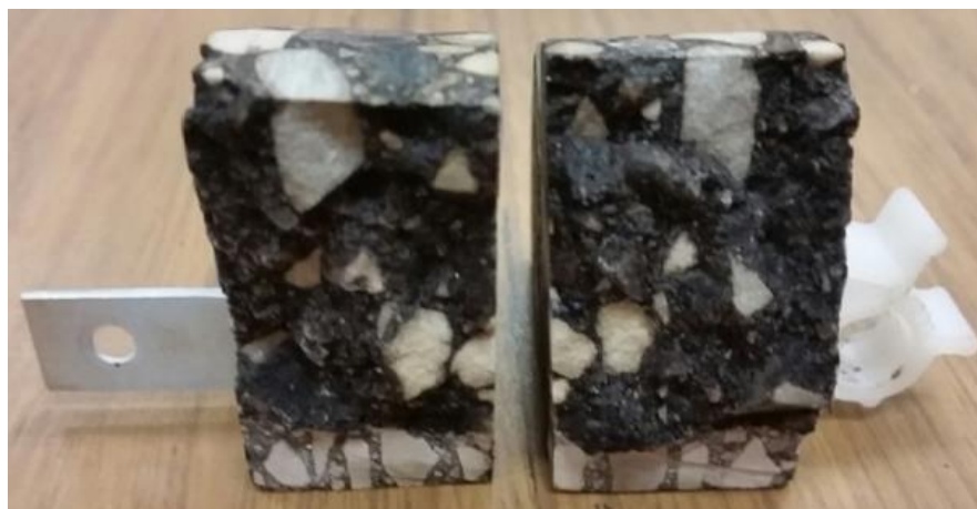
Figure 5.22 Representative Sample Failed in SCB
