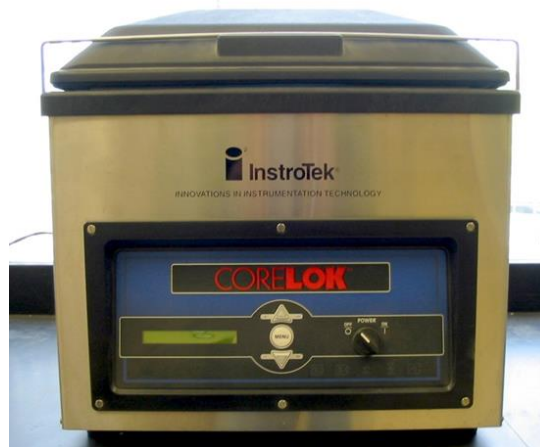
Figure 3.10 InstronTek CoreLok Machine used to Determine G_{mm} and G_{mb}
