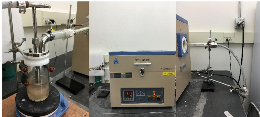
Figure 13. Photo for the spray CVD equipment.
