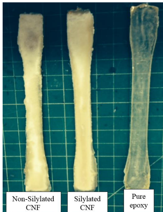
Figure 4. The CNF and pure resin specimens created for the tensile test.
