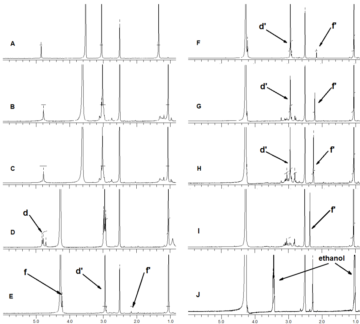
Figure 2-16. ^1\text{H} NMR analysis of 4b in deuterated DMSO, \text{D}_2\text{O} , and \text{H}_2\text{O}_2 : (A) ^1\text{H} NMR of 4b (0.003 mmol) in DMSO only; (B) 10 min in mixture of DMSO (300 \mu\text{L} ), \text{D}_2\text{O} (20 \mu\text{L} ), and pH8 buffer (10 \mu\text{L} ); (C) 2.5 h in mixture of DMSO (300 \mu\text{L} ), \text{D}_2\text{O} (20 \mu\text{L} ), and pH8 buffer (10 \mu\text{L} ); (D) additional 12 h after added additional DMSO (60 \mu\text{L} ) and \text{D}_2\text{O} (210 \mu\text{L} ) in C ; (E) 3 min after addition of \text{H}_2\text{O}_2 (3 equiv.) in D ; (F) 30 m after addition of \text{H}_2\text{O}_2 ; (G) 4 h after addition of \text{H}_2\text{O}_2 ; (H) 16 h after addition of \text{H}_2\text{O}_2 ; (I) 40 h after addition of \text{H}_2\text{O}_2 ; (J) Trimethyl amine ( \text{NMe}_3 ) in ethanol with addition of 1 M HCl (10 \mu\text{L} ).
