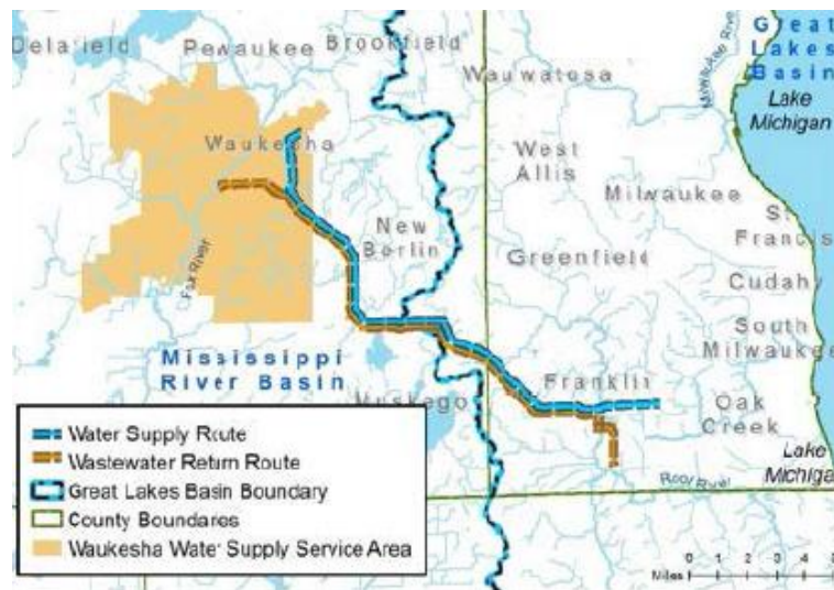
Figure 3. Current proposed diversion and return from Lake Michigan: Waukesha Wisconsin Diversion Application (WDNR 2015)
