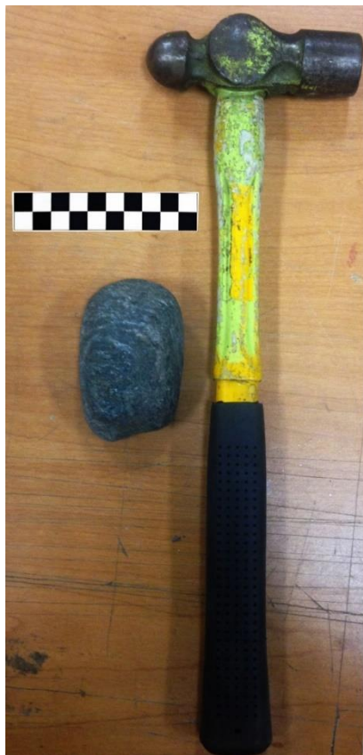
Figure 3.8 Granitic whetstone and ball-peen hammer used in cold hammering and sharpening each of the experimental sickles at the Milwaukee Makerspace.
