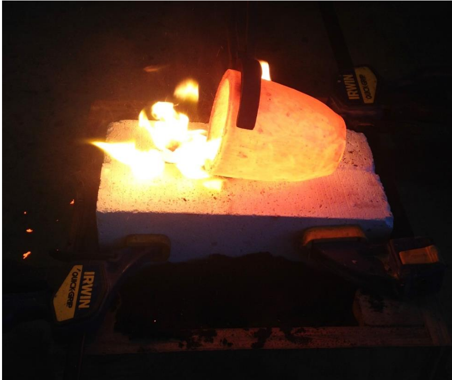
Figure 3.5 Pouring molten bronze into the fire brick mold.
