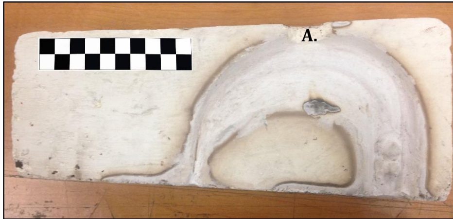
Figure 3.4 Completed fire brick mold ready for bronze pour.
