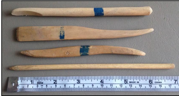
Figure 3.3 Wooden tools used for fire brick carving.
