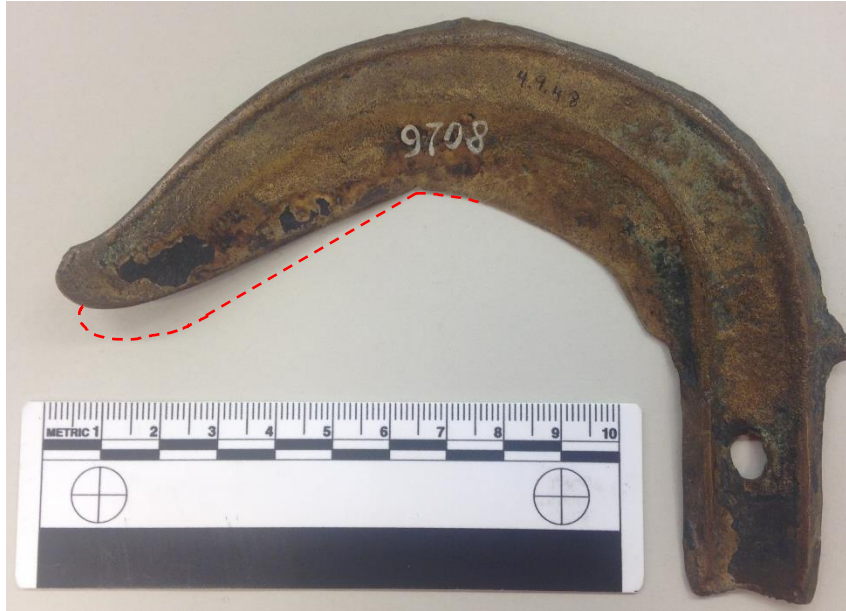
Figure 4.11 LM 4.9.48 showing warping of the sickle blade. The red dotted line outlines the shadowed area, revealing the warped nature of the blade.
