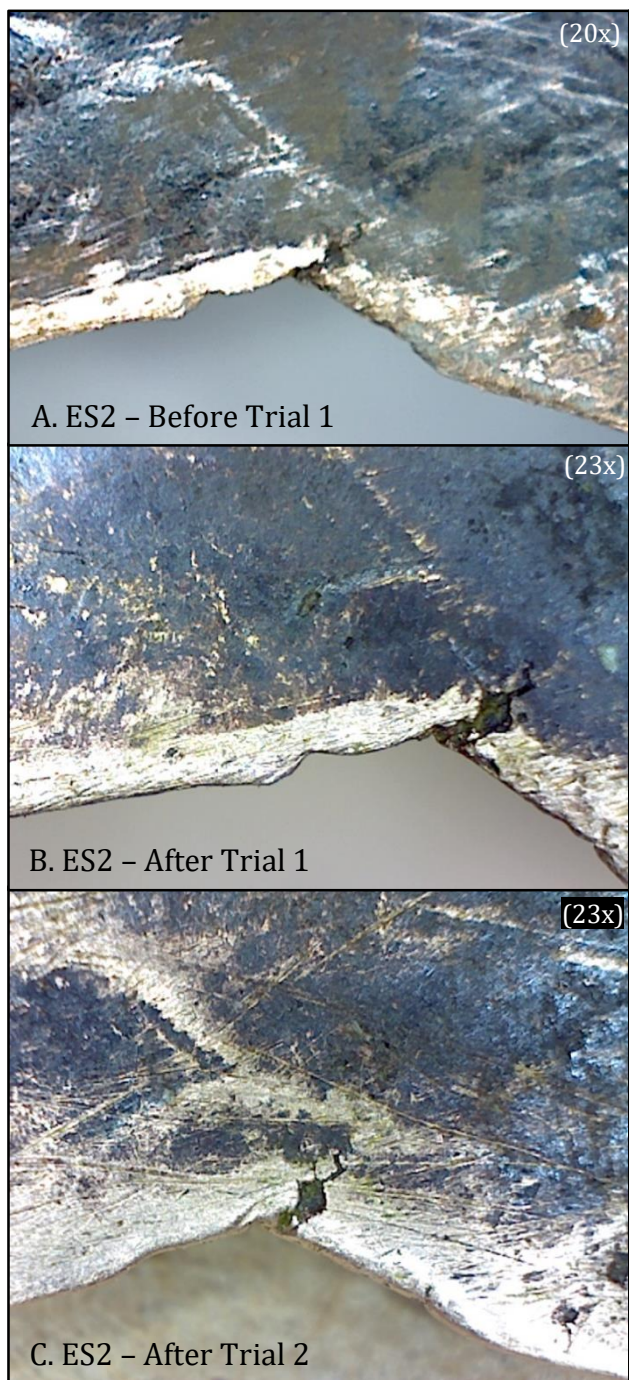
Figure 4.2 Microscopic images of a proximal area of Experimental Sickle 2 before and after trials. A. shows the control image with a sharp edge. B. shows the sickle after Trial 1 with a slightly rounded edge and slightly extended abraded area. C. shows ES2 after Trial 2 with a highly rounded edge and greatly extended area of abrasion. Image location is indicated in the dotted box on the sickle schematic above (D).
