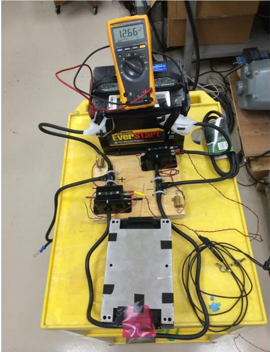
Figure 7.2. Balanced parallel connection Hybrid ESS.
