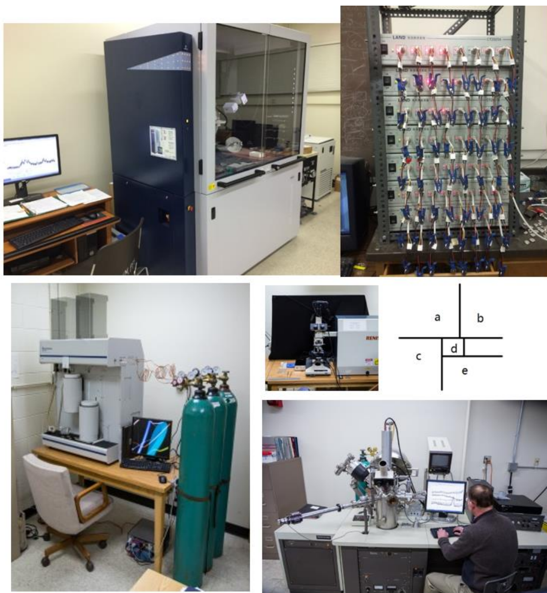
Figure 13(a). Bruker X-Ray Diffraction (b). Land battery testing system. (c). Micromeritics ASAP 2020 BET measurement. (d). Raman spectroscopy (Renishaw 1000B). (e). Perkin Elmer 5440 X-Ray Photoelectron Spectrometer.
