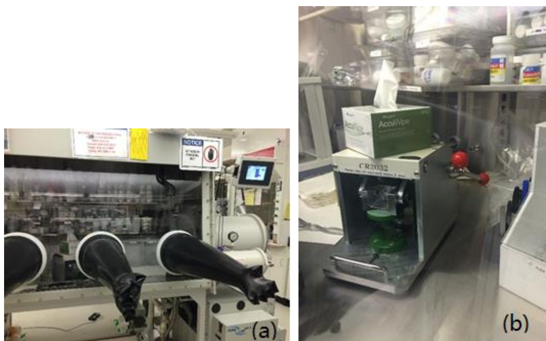
Figure 12(a). Glove box. (b). Hohson Corp HS-HCR2 manual coin crimper in glove box.
