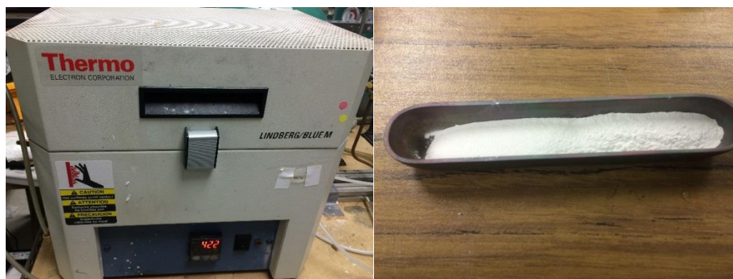
Figure 8(a). Tube furnace (Thermo Scientific Lindberg/Blue M™ Vacuum Ovens). (b). Samples became white powder after calcination
