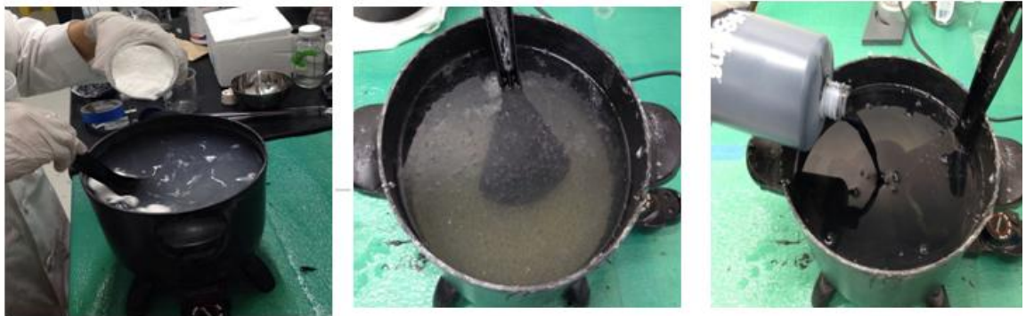
Figure 2-15: Black mounting medium preparation steps
