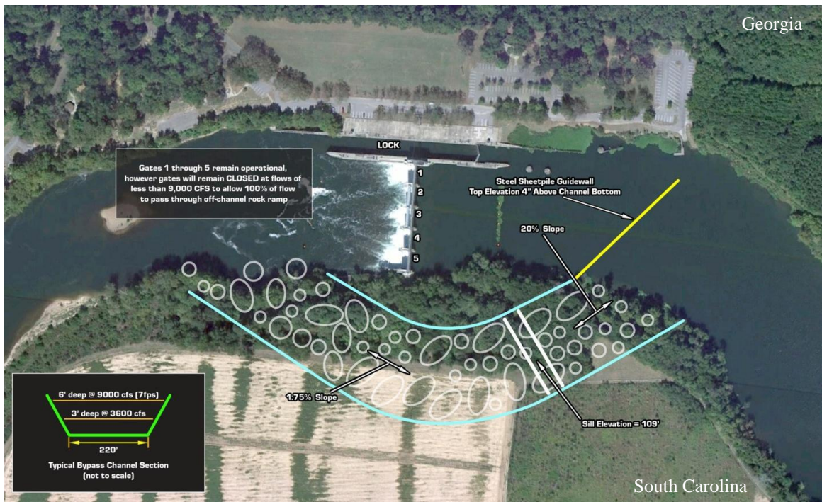
(Figure 6. Fish-passage at the New Savannah Bluff Lock and Dam. Source: U.S. Army Corps of Engineers 2012b, Appendix C p.75)
