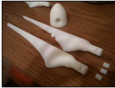
a. Straight and tubercle blade with hub and attack angle inserts
