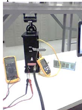
c. Calibrator used with Air flow meter and volt meter to construct calibration curve
