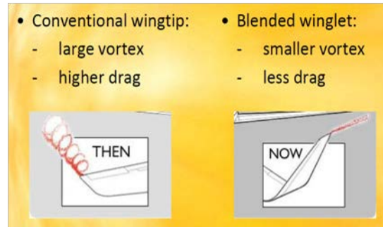
Figure 18: Reduction in the wingtip vortex size with the blended winglet.
