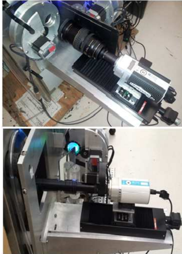
Figure 3.10: Macroscopy and Microscopy setups with moving stage for camera and lens.
