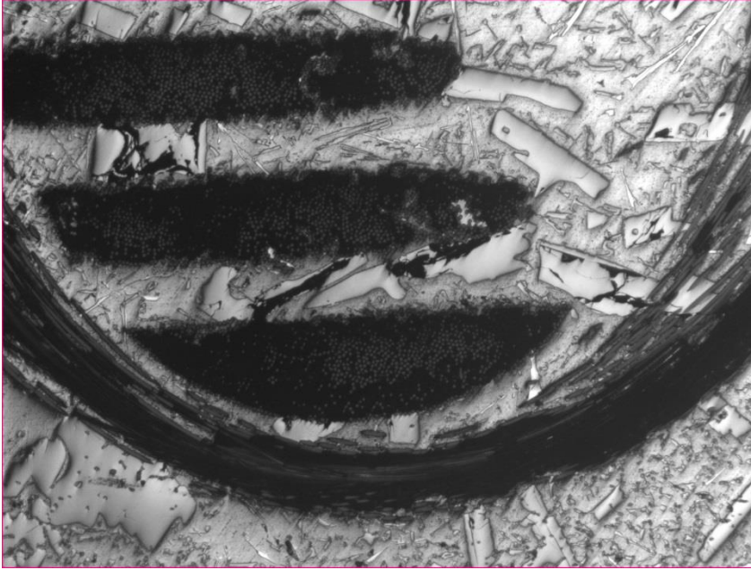
Figure 40. Micrograph of MMC with Mercusil Alloy as matrix made at 750C and 200 psi showing Z yarns (Magnification 50X)
