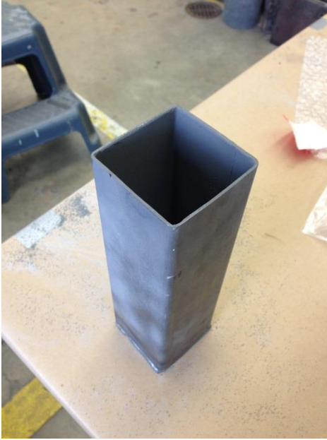
Figure 23. Square tube that was used as mold in the experiments.
