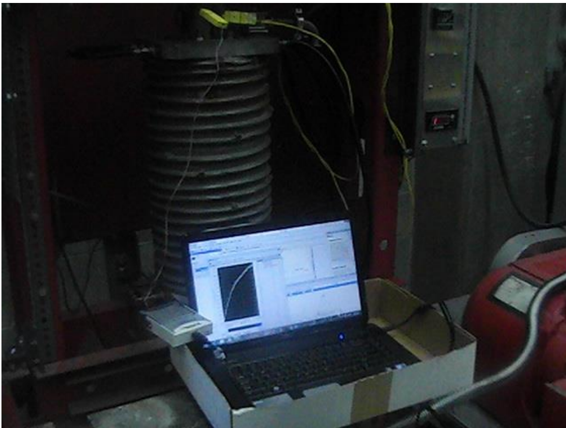
Figure 21. Labview Signal Express software was used to find the temperature map of the furnace.
