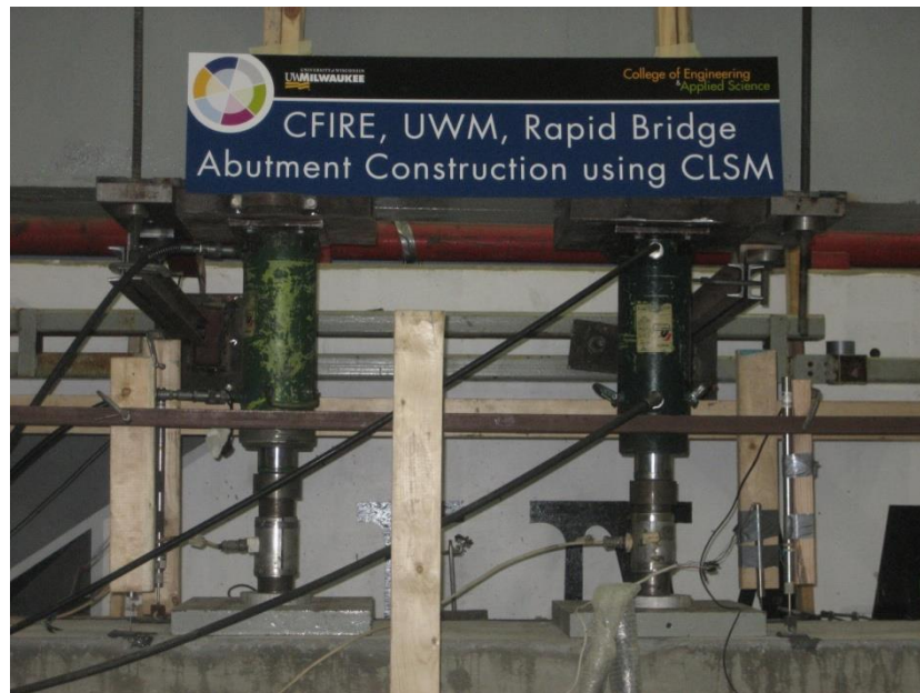
Figure 4.22: Two steel plates and hydraulic jacks on the bridge sill.
