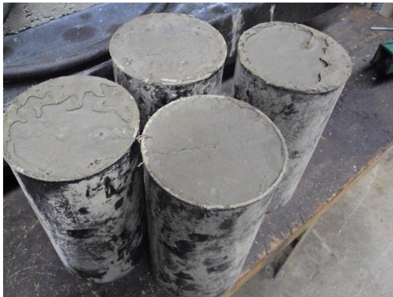
Figure 3.31: Collected samples from inside of the CLSM fill.
