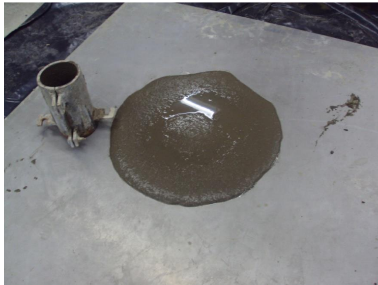
Figure 3.8: Flow cylinder test.
