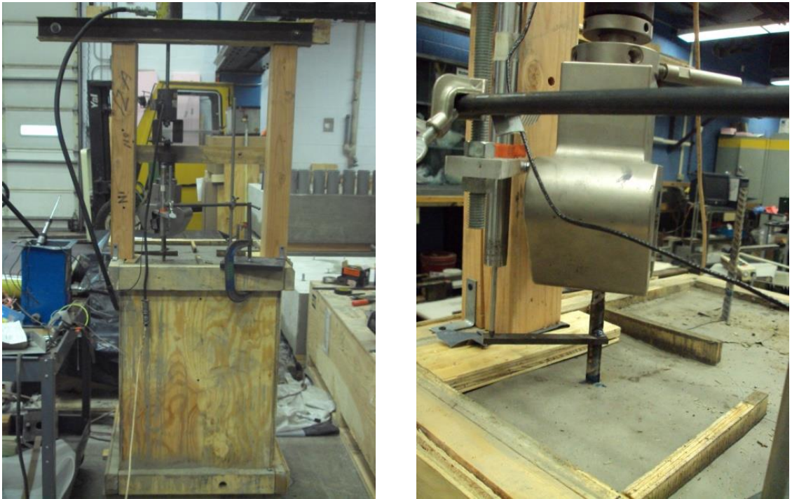
Figure 3.28: Large-scale pullout testing.
