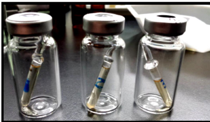
Figure 3-18. Photographs of: (a) NMR tubes sealed with glass, and (b) sealed NMR tubes in closed vials with the aged samples.
