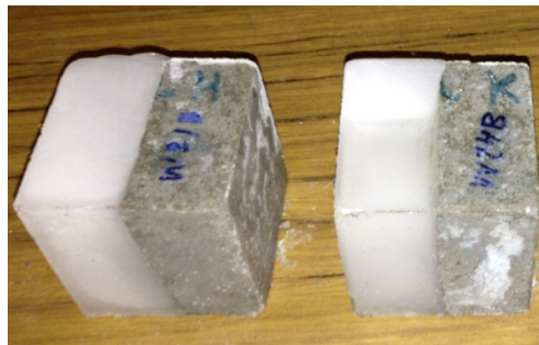
Figure 68. Coated and non-coated ice-concrete samples.
