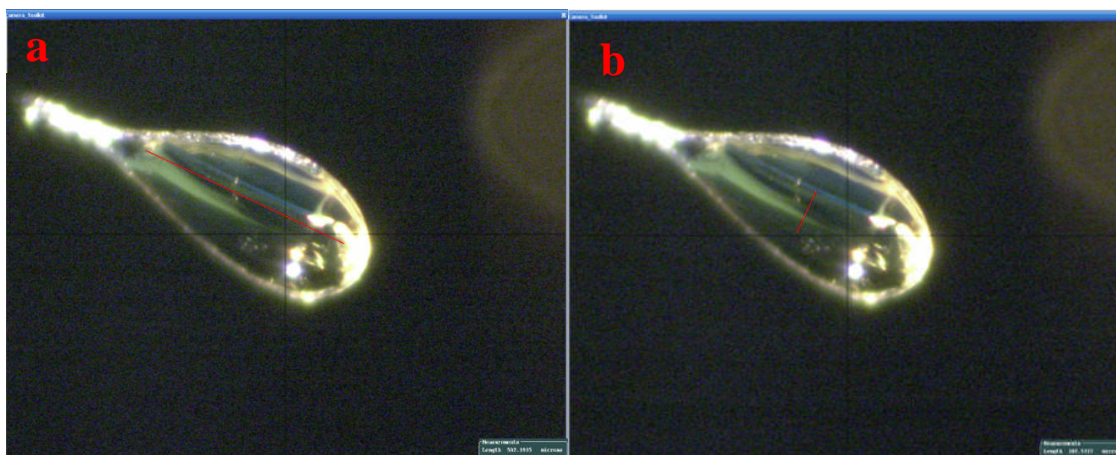
Figure 2-16: (a) Perfectly frozen crystal the length is 580mm (b) Perfectly frozen crystal the width is 185mm (screen shot).
