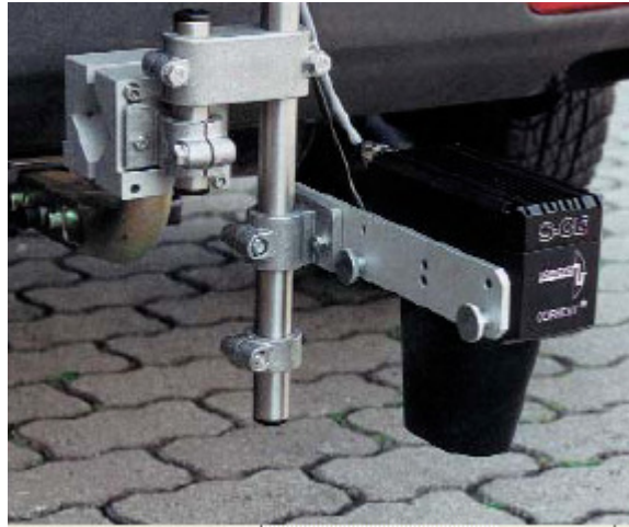
Figure 3-34: Contact-less optical sensor for measuring sideslip angle.
