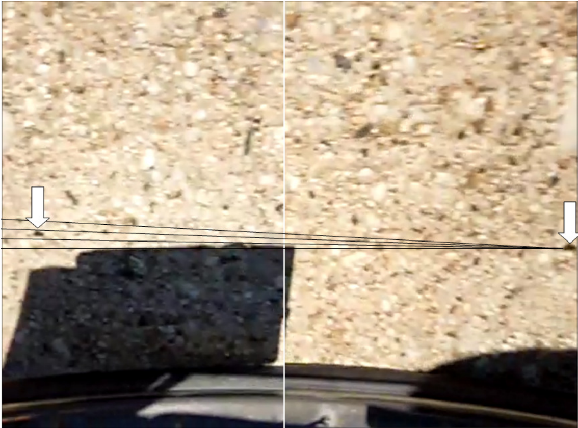
Figure 3-33: Extracting slip angle from sequential video frames.
