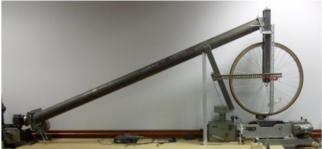
Figure 3-7: Photograph of test device number 2. The forward pivot is on the far left, and the flat-top chain track is under the wheel on the right.
