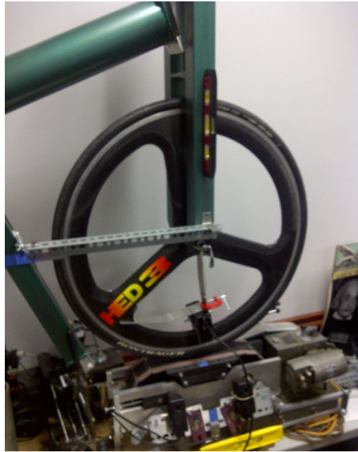
Figure 3-15: Measuring tire centerline lateral deflection on a HED Cycling carbon tri-spoked wheel.
