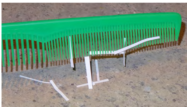
Figure 5.3 After being used to comb hair, this comb attracts small strips of paper from a distance, without physical contact. Investigation of this behavior helped lead to the concept of the electric force.
