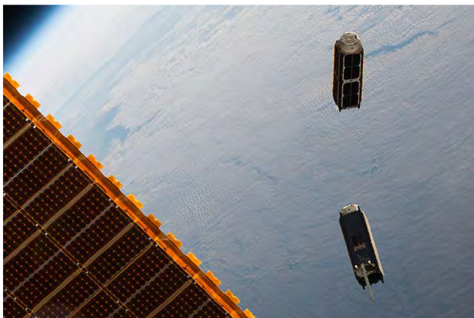
Figure 16.16 Two small CubeSat satellites deployed from the International Space Station in May, 2016. The solar sails open out when the CubeSats are far enough away from the Station.
