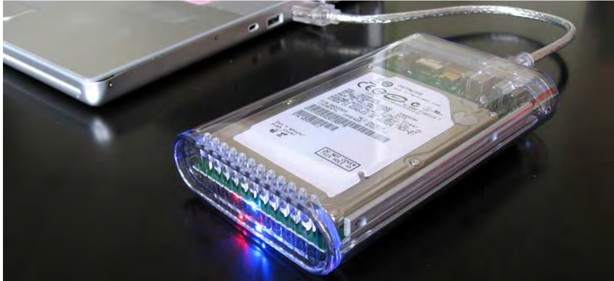
Figure 12.1 An external hard drive attached to a computer works by magnetically encoding information that can be stored or retrieved quickly. A key idea in the development of digital devices is the ability to produce and use magnetic fields in this way. (credit: modification of work by “Miss Karen”/Flickr)
