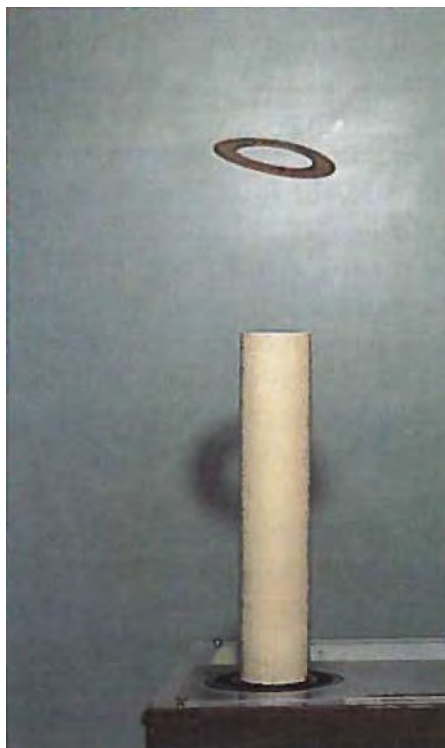
Figure 13.10 The jumping ring. When a current is turned on in the vertical solenoid, a current is induced in the metal ring. The stray field produced by the solenoid causes the ring to jump off the solenoid.
