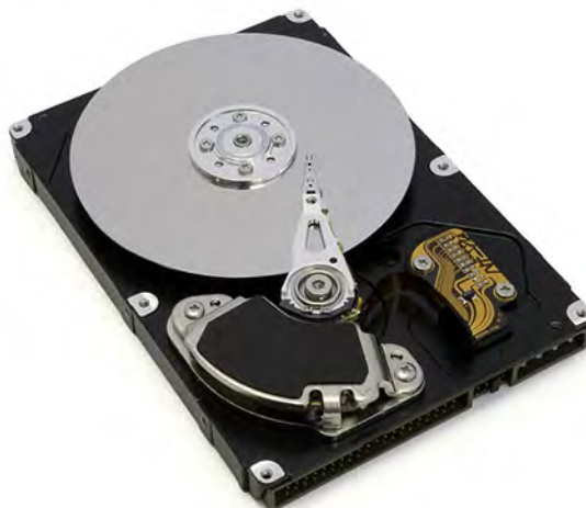
Figure 12.28 The inside of a hard disk drive. The silver disk contains the information, whereas the thin stylus on top of the disk reads and writes information to the disk.
