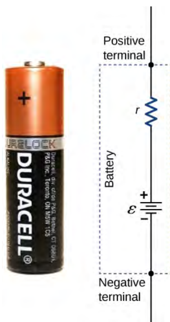
Figure 10.6 A battery can be modeled as an idealized emf ( \epsilon ) with an internal resistance ( r ). The terminal voltage of the battery is V_{\text{terminal}} = \epsilon - Ir .
