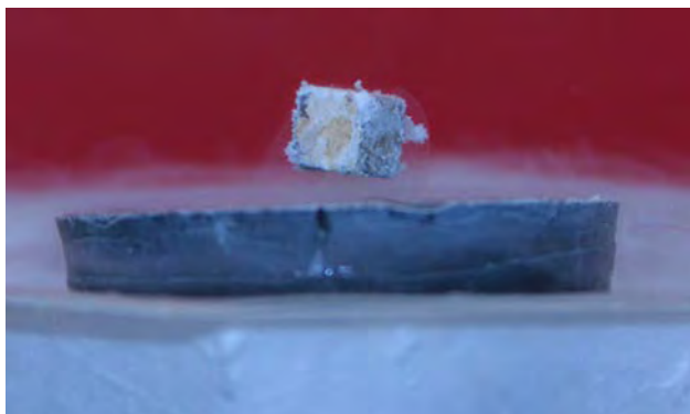
Figure 9.28 A small, strong magnet levitates over a superconductor cooled to liquid nitrogen temperature. The magnet levitates because the superconductor excludes magnetic fields.
