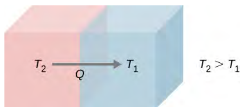
Figure 4.3 Spontaneous heat flow from an object at higher temperature T_2 to another at lower temperature T_1 .
