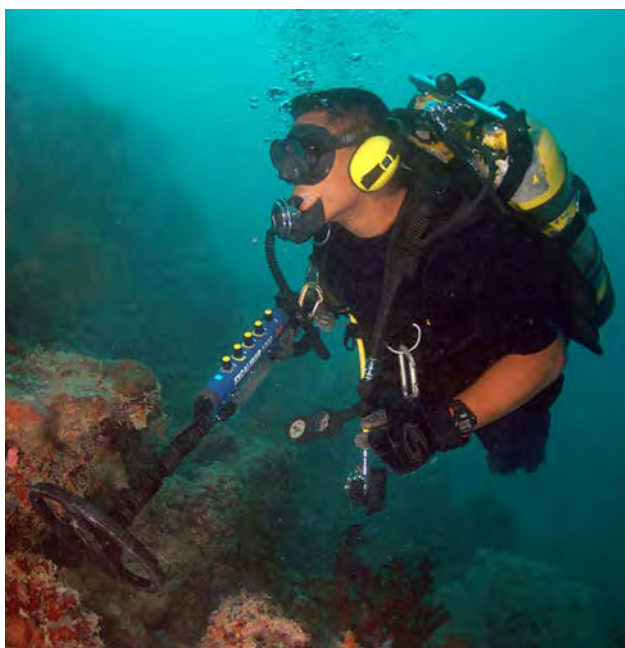
Figure 15.19 When a metal detector comes near a piece of metal, the self-inductance of one of its coils changes. This causes a shift in the resonant frequency of a circuit containing the coil. That shift is detected by the circuitry and transmitted to the diver by means of the headphones.
