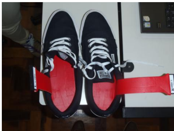
Figure 42. pressure distribution Insole that measured the ground reaction force for each subject.
