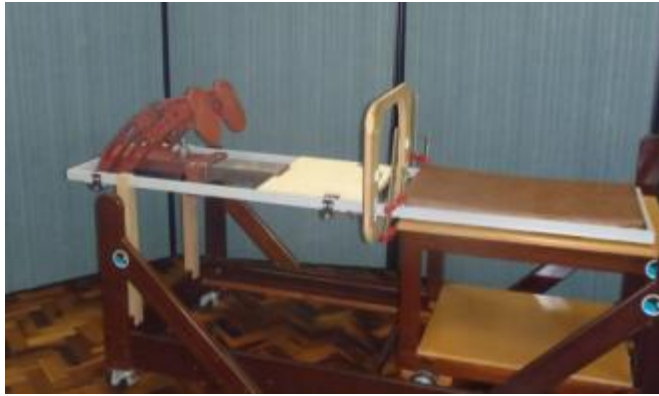
Figure 46. second prototype mated to the existing trolley, shown on the left, after the horizontal supports were relocated. The 2nd prototype mated to the existing LBNP box, shown on the right.
