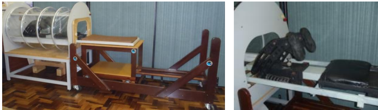
Figure 10. The left photo shows final integration of the multi-platform to the existing LBNP Box. The right photo displays a close up of the multi-platform outside of the LBNP Box.
