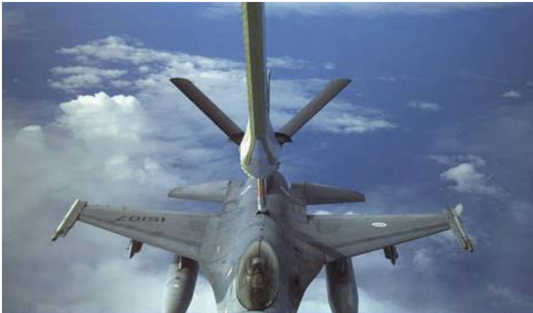
Figure 2, Boom re-fueling systems.
