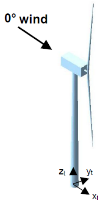
Fig. 5.3 Tower-base Coordinate System [140]
