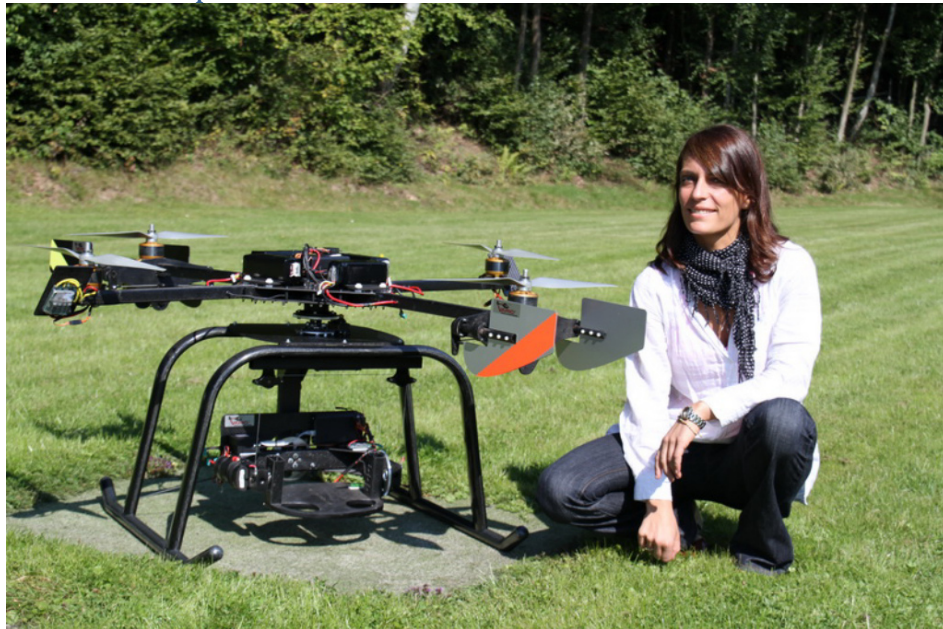
Figure 8: The usage capabilities are widespread. As seen here, this quadcopter type UAS can be mounted with a variety of sensors such as cameras, infrared detection systems, or other analysis tools.
