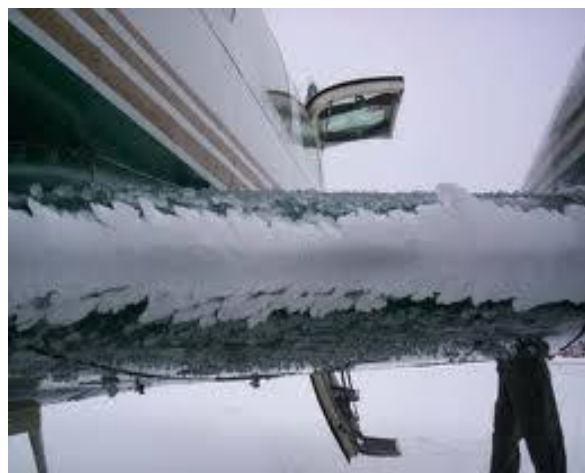
Figure 4: leading edge ice build-up on a wing.
