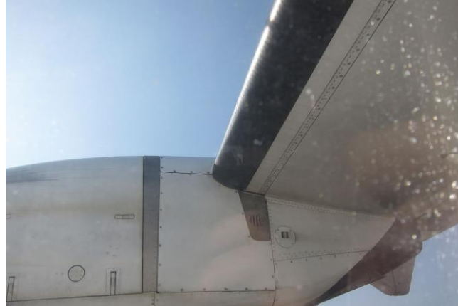
Figure 3: rubber leading edge ice removal mechanism.
