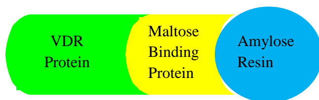
Figure 46: Maltose binding protein (MBP) attached to an amylose resin. MBP is a member of the maltose and maltodextrin system of E. Coli , which is responsible for the catabolism of maltodextrins. Maltose can be immobilized by cross-linking to a solid-support amylose resin. The purified MBP fusion protein can be dissociated and eluted by the addition of excess maltose (10 mM).
