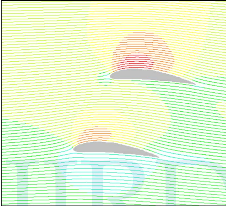
Figure 11. Flow distribution with positive stagger.
