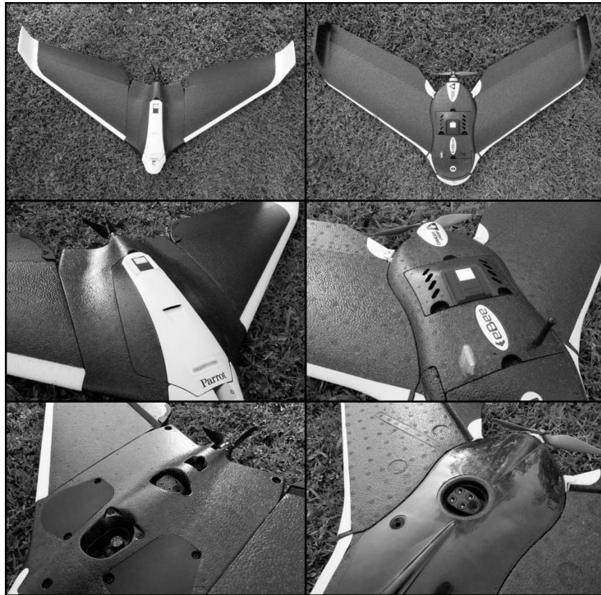
Figure 1. Image comparisons between the Parrot Disco Pro Ag (left column) and the senseFly eBee (right column). De Leon Springs, FL. February 21, 2018.
