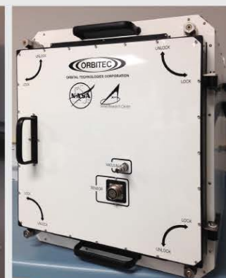
PMWC (Plastic Melt Waste Compactor) Melt Chamber
