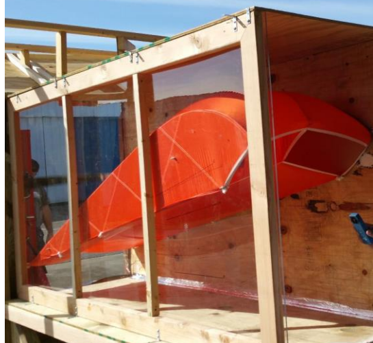
Figure 2.27 Experimental test of a single cell canopy. Adapted from (Burnett, 2016).
