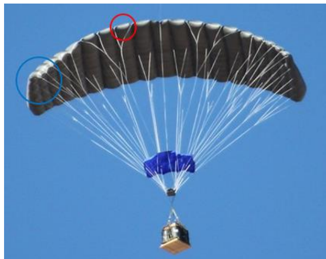
Figure 2.2 Rear view of an inflated ram-air parachute (Adapted from Air Freshener, retrieved from https://airfreshener.club/quotes/ram-air-parachute-dimensions.html )
