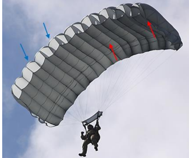
Figure 2.1 Underside view of an inflated ram-air parachute (Adapted from Tactical Parachute Delivery Systems Inc., retrieved from http://tpdsairborne.com/products/parachutes/hlt-r/ )
