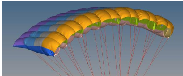
b) Deformations of the canopy structure caused by external surface pressure, variation along the chordwise direction.
