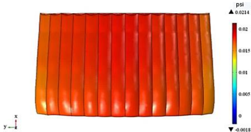
Figure 2.22 Internal surface pressure for the seven-cell canopy at 0^\circ angle of attack, top view. Adapted from (Fonseca, 2018).
