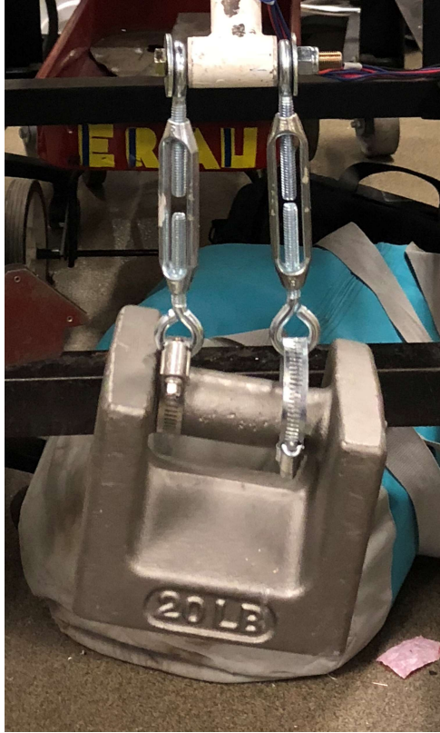
Figure 39: Weight Balance for Strain Gauge Axial Calibration Utilizing Two Turnbuckles.
