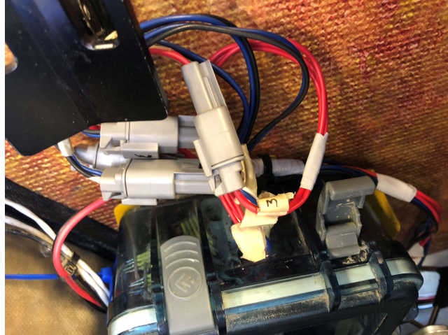
Figure 33: Wire Harness Connected to DAQ Box
