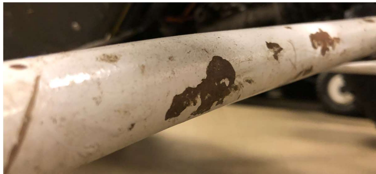
Figure 21: Control Arm Deformation Area, Enhanced
