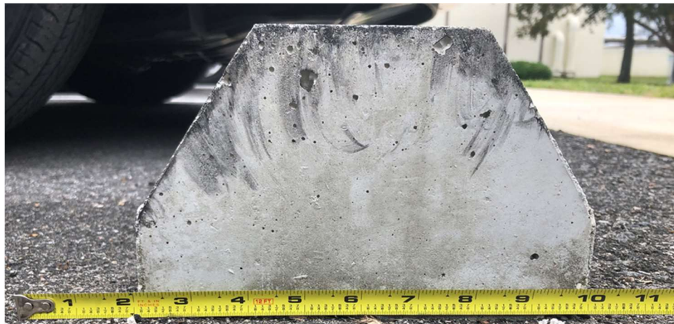
Figure 26: Parking Chalk Width Measurement
