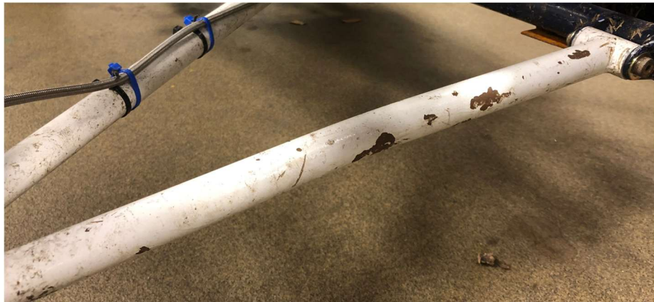
Figure 20: Right Front Lower Fore Control Arm, Deformation
