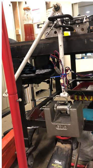
Figure 38: Strain Gauge Calibration Setup for Axial Loading, Along Positive y-axis.
