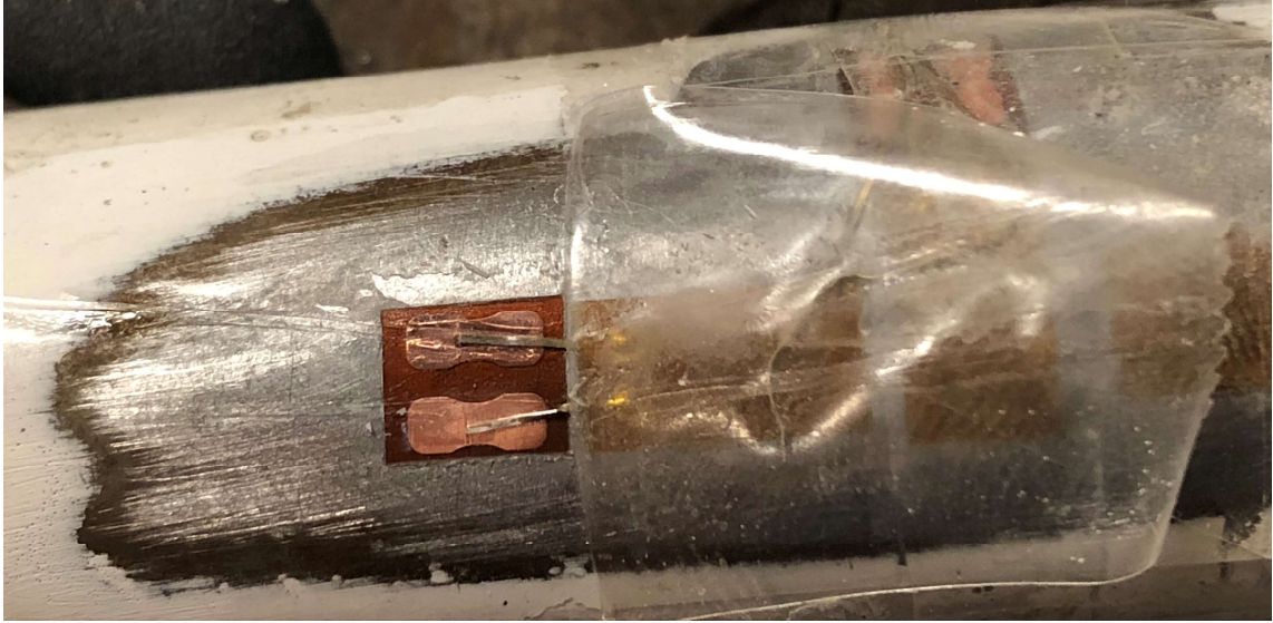
Figure 50: Ribbon Leads Aligned on Solder Pad with Protective Coating Removed.
