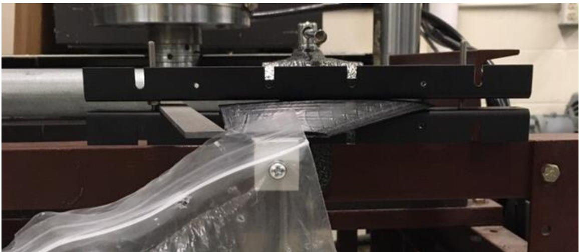
Figure 5.5 3D printed F-5 wing fixture
