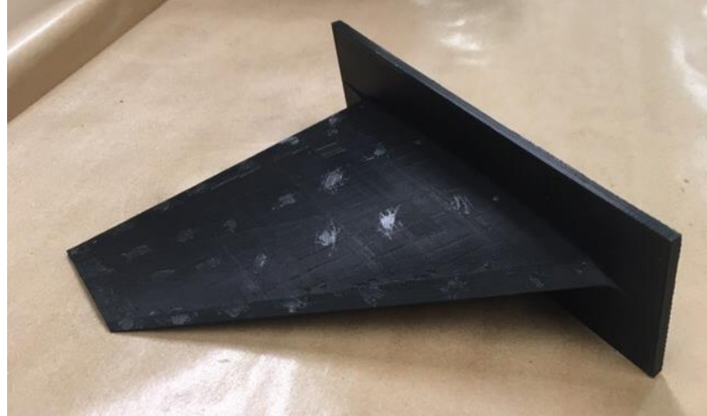
Figure 5.15 3D printed wing with a flange
