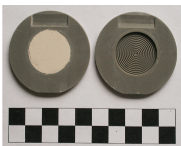
Figure 4.54. Sample holder used for dry powder diffraction (left with sample, right empty).
