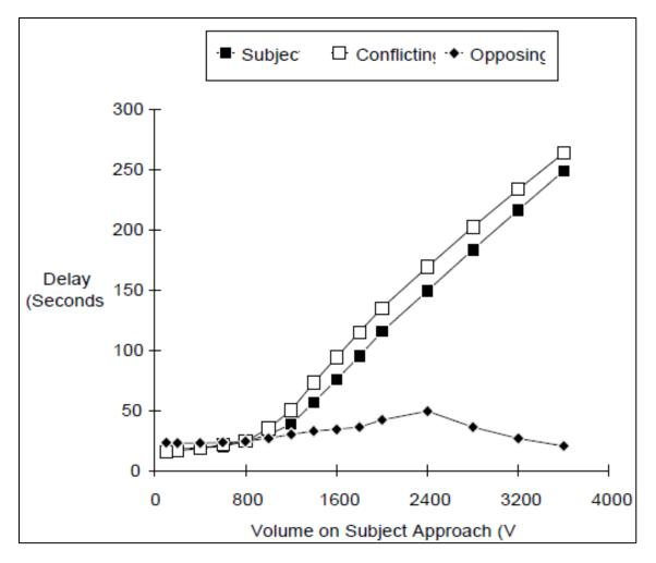
Figure 2: Approach Volume Verse Delay (Horowitz, Delay/Volume Relations for Travel Forecasting Based upon the 1985 Highway Capacity Manual, 1991)
