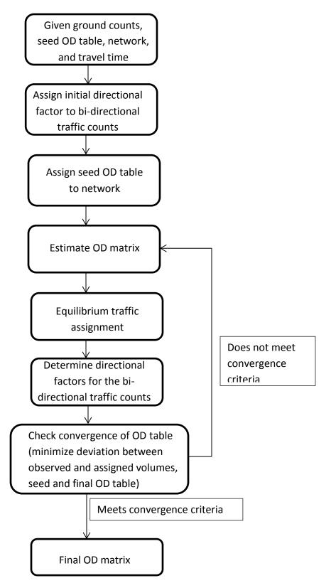
Figure 5 OD estimation using Travel Time to Set a Directional Factor for Bi-Directional Traffic Counts.
