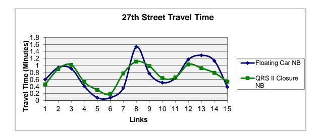
Figure 20: Travel Time Comparison showing Individual Link Travel Time between Floating Car and QRS II with Closure
