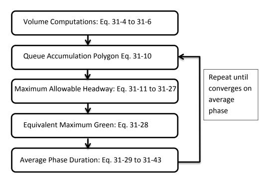
Figure 3: Step from the 2010 HCM for Calculating Average Actuated Phase Duration
