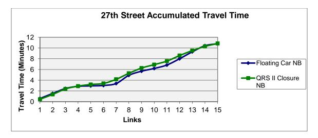
Figure 21: Travel Time Comparison Showing Accumulated Travel Time in a Corridor The above figures show that although 27<sup>th</sup> Street travel time is comparable between floating car data and QRS II modeled when averaged over a corridor, the individual length segments are considerable deviations.
