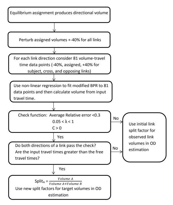
Figure 9: Procedure for Calculating Directional Factors for Observed Bi-directional Ground Counts
