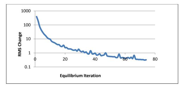
Figure 12: The link RMS change from previous equilibrium iterations using actuated signals
