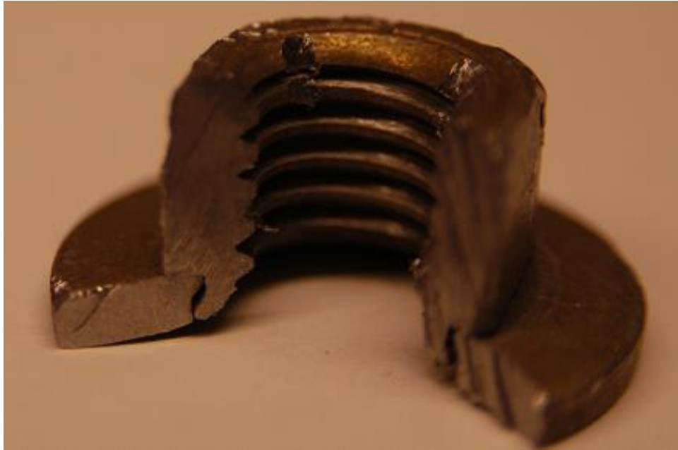
Figure 2-3. Macro Photograph of Sectioned Nut and Integral Washer.
