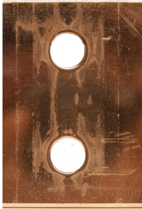
Figure 3-8. Mating Surface where Power Conducting Bus meets Load Bus
