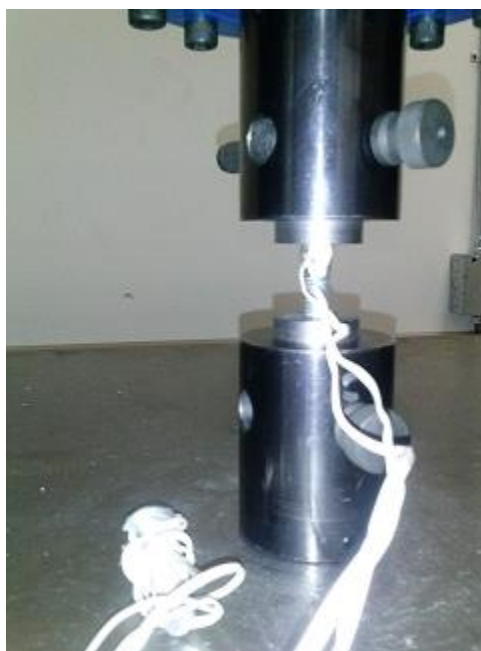
Figure 2-16. Detail View of Load Cell in Grips.
